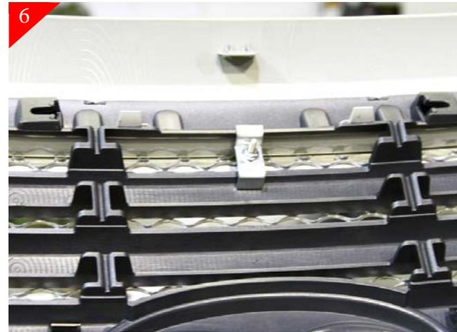
Locate the 3 upper supplied brackets shown above. Place brackets as shown and attach until just snug with 10-24 nyloc nuts. **Again do not fully tighten until you have all brackets in place and have checked alignment.**
