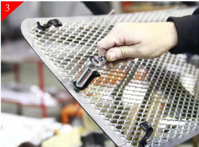
Now attach 3 brackets to the outside drivers side mounting studs using the 10-24 nyloc nuts align brackets as shown. Repeat for the 3 brackets for the passenger side of mesh.
