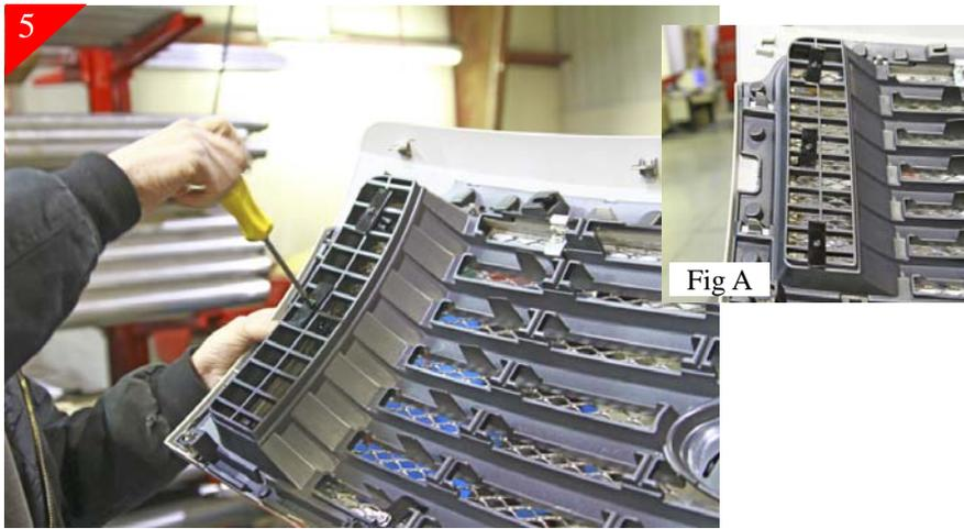
Now attach tabs to the already placed brackets as shown above. Get all the tabs in place and tighten just until snug. This will hold mesh and trim ring in place while you place the remaining brackets. **Again do not fully tighten until you have all brackets in place and have checked alignment.**
