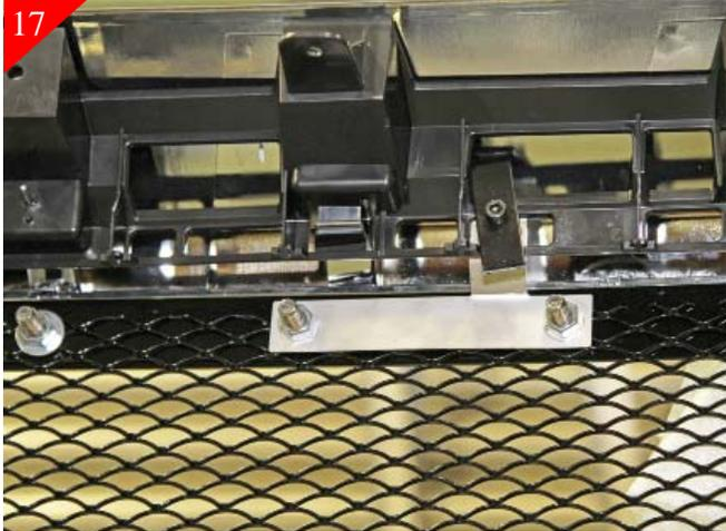
Moving to the upper brackets attach bracket using supplied rectangle tab and 1/4-20 x 5/8" bolt and 1/4-20 nuts as shown above.
