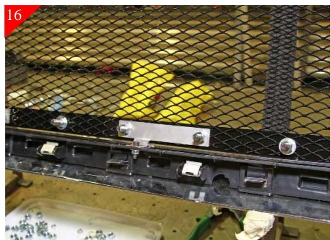
Place grill back into opening and center. Now you will be attaching mesh to stock grill shell. Starting with the (4) outside corners replace the removed bolts from step 13 and tighten. Next place 1/4-20 x 5/8" bolt through the bottom brackets and secure with 1/4-20 nut repeat for remaining bottom bracket.
