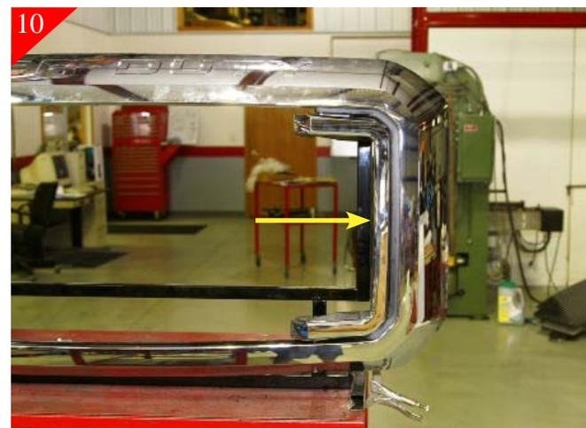
Turn grille shell over face up. Using a cut-off wheel you will be removing the inner chrome portion shown above.
