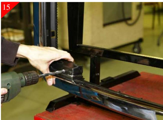
Next remove grille from opening and drill all just marked hole locations using a 1/4" drill.
