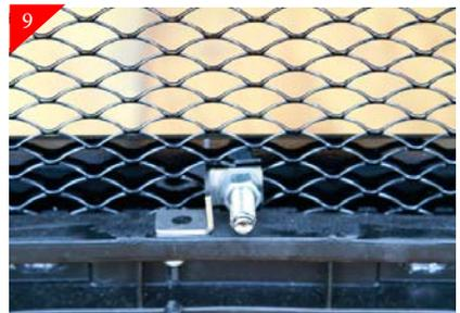
Loosen bolts that are holding the brackets in place. Next place the mesh grille into opening and center and rotate the brackets so that they meeting up with the stock shell. Check alignment and mark all brackets using a scribe or sharpie.
