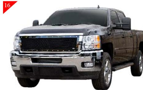
With mesh grille secured to the stock grille shell. Attach stock grille shell back on vehicle.
