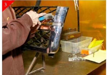
Now you will be removing the center portion of the stock grille shell. Following the black plastic as a guide cut or trim cross hatch center where it meets the outer most of the grille shell.
