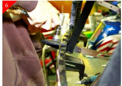
Using a sanding block sand all cut areas smooth with shell.
