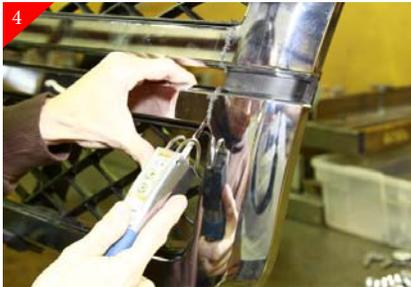
When you get to the Chrome bar that run through the center of the stock grille shell. You will need to cut straight down and then continue to follow the black plastic as a guide. Continue on around so the center will be free.
