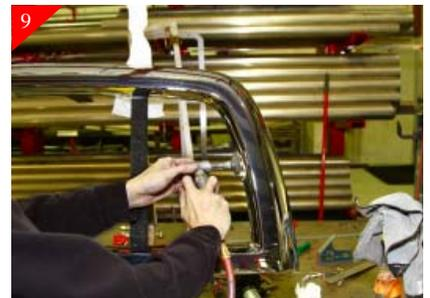
Using a grinder or sanding block sand all cut areas smooth with shell.
