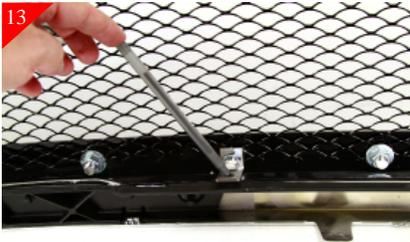
With all brackets attached place mesh grille into opening and center. Using a couple pair of vice grips check alignment of mesh grille and clamp the backside of the grille shell and brackets. This will aid in holding the mesh in place while marking hole locations. Next you will mark hole locations of the just placed brackets.
