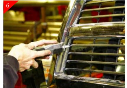
Continuation of Step 5 cutting vertical and horizontal attachment points.
