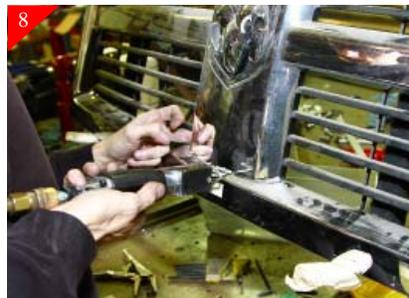
Continuation from step 7 cutting large vertical and horizontal attachments. After cutting grille center will be free at this point and can be removed.
