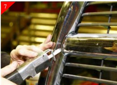
Now you will be removing the larger attachment points. Using an air saw/cut-off wheel cut the large chrome plastic vertical and horizontal attachment points leaving enough material to come back and finish sand.
