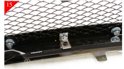
Place mesh grille back into opening and center attach brackets using the supplied 1/4-20 head bolts and 1/4 nuts as shown above. Repeat for all remaining brackets.
