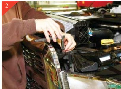
Remove the 10mm bolts holding top portion of the stock grille shell in place.
