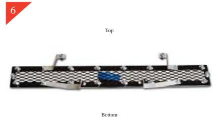
Remove mesh bumper grille from packaging. All necessary brackets and hardware will already be attached to mesh grille in the correct locations as shown.
