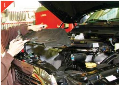
Start with removing the plastic push pull style rivets hold core support cover in place. Remove core support cover.
