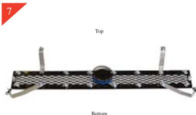
Loosen nuts that are holding brackets in place. The brackets are rotated in for shipping purposes. Next you will remove the bolts and nuts from opposite end of brackets. Rotate brackets as necessary to place mesh grille into bumper opening and center. Then rotate brackets similarly as shown above.
