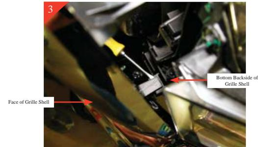
With the top portion of grille shell free, pull shell forward so you are able to reach down the backside of grille shell to release clips holding bottom portion of the stock grille shell in place. Using a regular screwdriver pry up to release clips.
