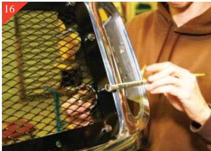
Place center portion of mesh grille into opening and center. Remove the 2 bolts that line up with the holes drilled in step 13. Secure the mesh in place with the bolts just removed.
