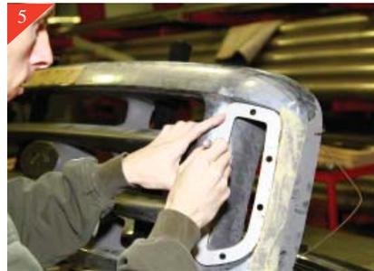
5 Next locate the correct side pocket mesh grille ring. Using the ring as a pattern place into the opening and center. Using a sharpie mark the hole locations.
