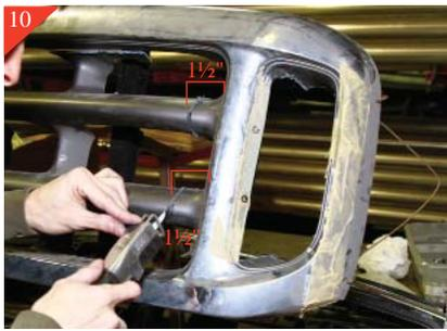
Cut the horizontal attachment points as shown. Show above is the right side portion of the stock grille shell. Repeat for opposite side.
