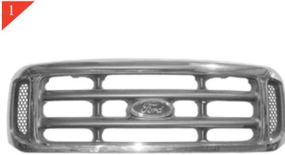
1 Remove core support cover and screws from top of grille shell. Release 4 spring clips at bottom of grille using flat blade screw driver. Remove grille shell from vehicle.
