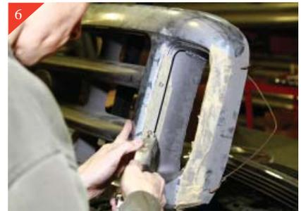
6 Using a sharpie mark a cut line as shown above. Make sure to cut around the just marked holes. These will be used in mounting brackets. Cut using an air saw or cut off wheel. Repeat for opposite side.
