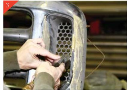
3 Next you will remove the egg create portions of the left and right pocket on stock grille shell. Remove using a air saw/cut off wheel using the inside of the opening as a guide. Repeat for opposite side of shell.
