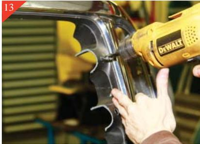
Using a 3/8" drill bit drill the just marked locations. Repeat for opposite side. Using the marked holes from steps 5 & 6 go ahead and drill these marked locations as well.
