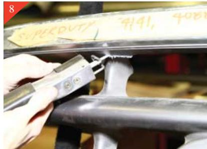
8 Next you will be removing the center portion of the stock grille. Using a air saw/cut-off wheel. Cut the vertical attachment points as shown. Show above is the top portion of the stock grille shell.
