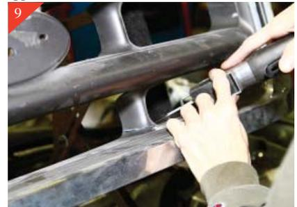
9 Cut the vertical attachment points as shown. Show above is the bottom portion of the stock grille shell.
