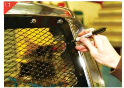
Place mesh grille into opening and center. Using a sharpie mark the 2 hole location as shown above. Repeat for opposite side. After marking remove mesh grille from opening.
