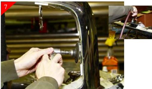
Using a grinder/sanding block sand all cut areas smooth with grille shell.
