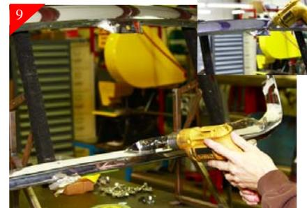
Using a 3/8" drill bit drill the just marked location from step 8 top and bottom.
