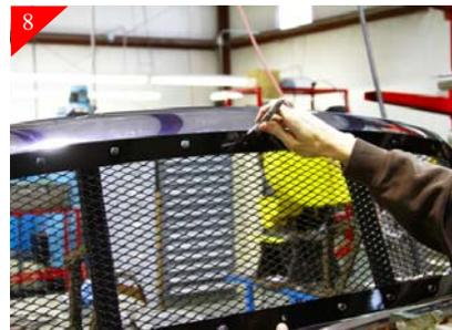
Place the mesh grille into opening and center using a sharpie mark the top and bottom center hole as shown. Remove grille from opening.
