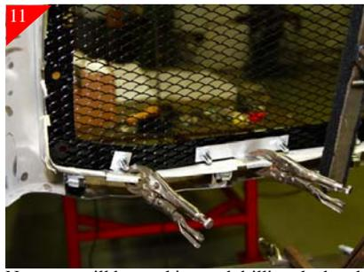
Next you will be marking and drilling the bracket locations. Starting with the bottom brackets. locate the small outer brackets and loosen the bolt and nut in order for it to catch the back side of the stock shell then tighten until snug repeat process for all the bottom brackets.
