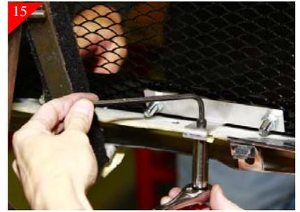
Place mesh back into opening and center. Loosen if necessary brackets so that they will catch backside of stock grille. Using the supplied 1/4-20 x 5/8" soc head bolts and 1/4-20 nuts secure the brackets in place.
