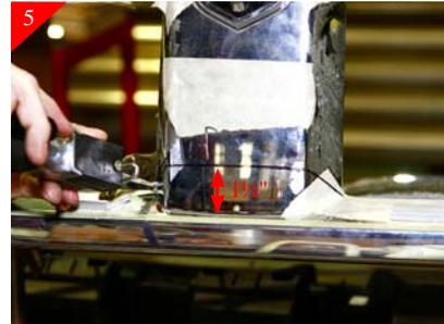
Next you will be cut/remove the center post. Start by using a sharpie to make a cut line. Measure up 1 1/2" and make a straight line across the post then for the side cuts angle to the backside of the grille shell.
