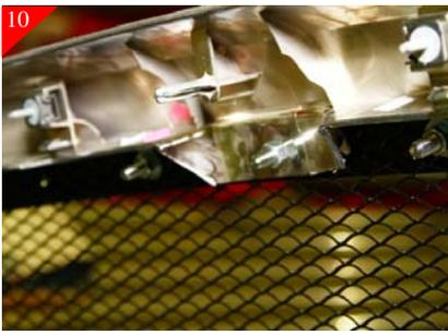
Place mesh grille back into opening and place supplied 12point bolt into just drilled locations top and bottom place a washer on backside followed ny nut tighten to hold in place.
