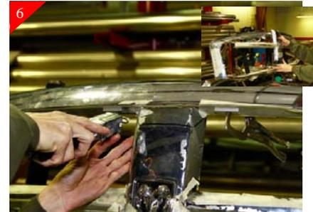
Using same cut procedure as previous step. Measure down 1 1/2" Make a cut line using a sharpie and cut. Center portion of grille shell will be free at this point.
