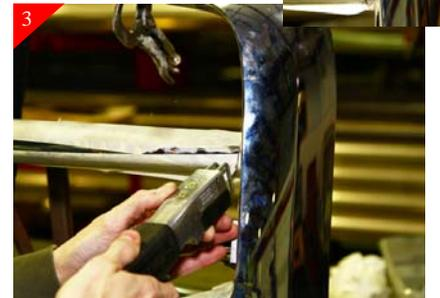
Next you will be removing the center portion of the stock grille. Start by using an air saw or cut-off wheel starting on the right side cut as shown above. Leave enough material so you can come back and finish sand all cut areas.
