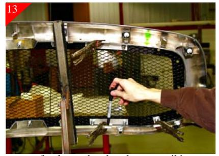
Repeat process for the top brackets loosen until it catches the back side of stock grille shell tighten until snug. With all brackets in place using a sharpie mark all bracket location.
