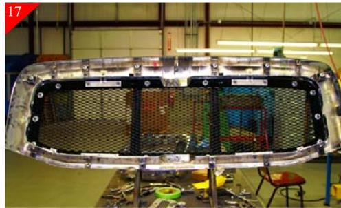
Backside of shell with all brackets attached.
