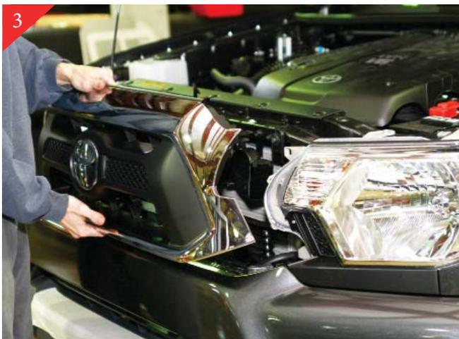
With top portion of shell free. Locate clips along bottom of stock shell and release. Do so by lifting up on the tabs to release. Stock grille shell will be free at this point.
