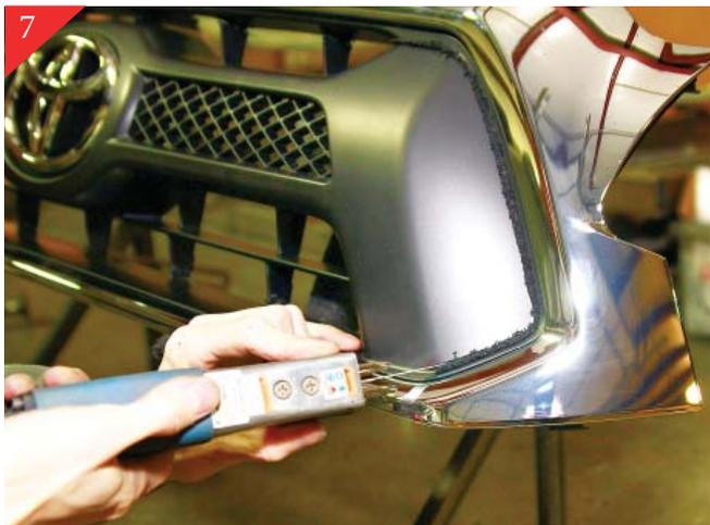
Continued Cutting of Shell from step 6. Again making sure not to cut into the chrome portion of stock shell.
