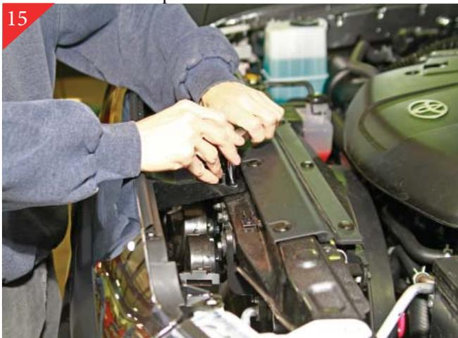
Place shell back on vehicle. Snap the bottom portion of the grille shell in place followed by the (2) 10mm bolts and (2) plastic rivets. Ref steps 1-3
