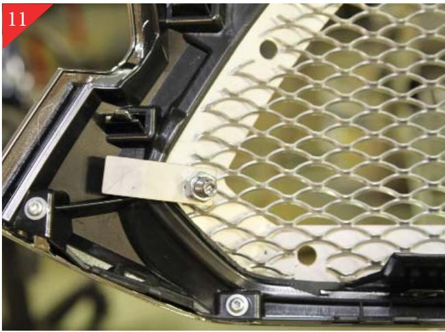
Place grille into opening and center. Using the (2) outer brackets place as shown. This allows the grille to stay in place as you to mark hole locations for drilling and mounting.
