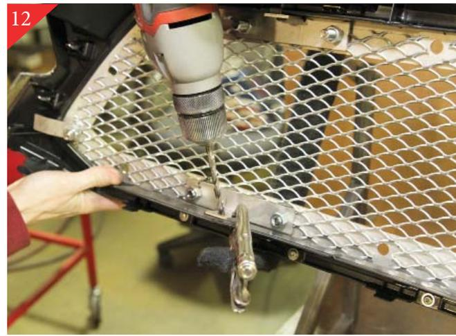
Also if necessary use a pair of vice grips to clamp bracket in place while marking holes. Check alignment across the face of the grille make any adjustments. Then using a scribe mark hole locations. Now using a 1/4" drill bit, drill the just marked locations. You may remove the grille during drilling. Repeat process for all (4) mounting brackets.
