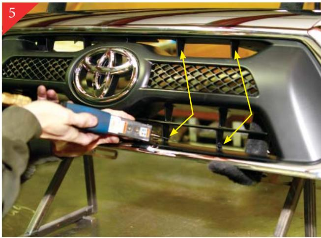
Using a air saw or cut-off wheel cut all the plastic vertical attachment point leaving some material for finish sanding. There are 5 attachment points for the top and bottom.
