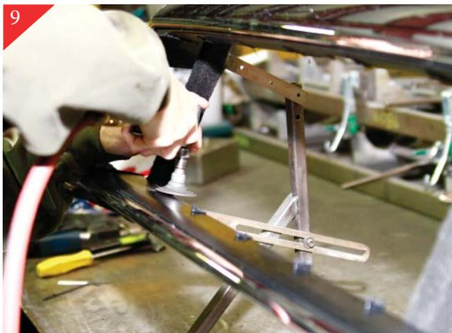
Next using a sanding block or air sander sand all cut areas smooth with the stock shell as shown.
