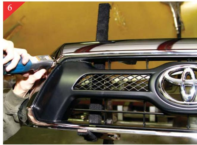
Using the black plastic where it meets the chrome portion of the shell as a guide cut with air saw without cutting into the chrome. Making sure to leave enough material for finish standing.
