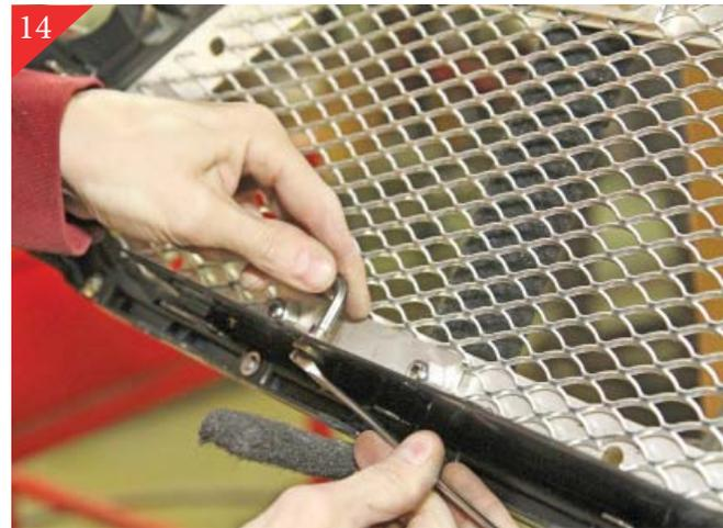
Mounting of the bottom portion of the grille. Place supplied 1/4-20 x 5/8" allen bolt through bracket and shell then place supplied washer followed by 1/4-20 nut and secure.
