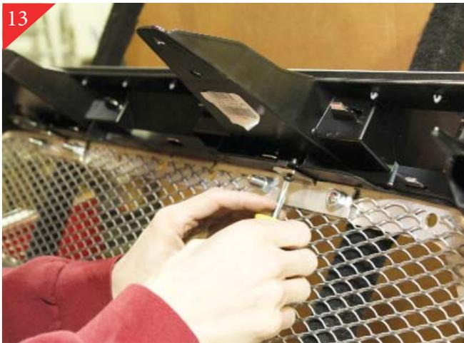
Start with mounting the top of the grille. Place supplied 10-24 u-clips on the top 2 mounting holes that were just drilled in step 12. Then attach using the supplied 10-24 x 5/8" phillips pan head screws. Secure in place
