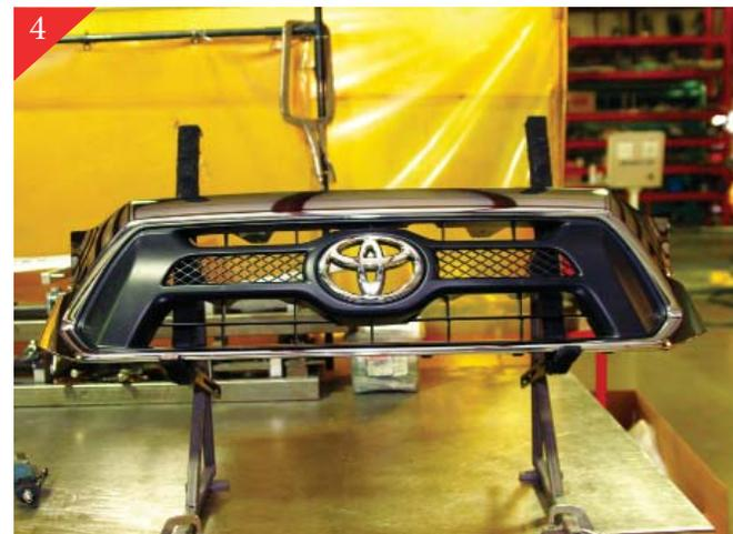
Move shell to a protective work surface. Also tape chrome portion of stock grille shell to protect during installation.
