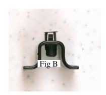
Start by placing the "Barrel Clip" into hole opening in bracket as shown above (Fig B.). Next center the emblem on the billet grille making sure that the emblem is correctly located. Place the brackets on the backside of the billet grille and simply push the emblem and the bracket together as shown in the diagram below.
