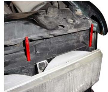
**3.** Remove the vertical rods on outside and near the center holding the headlamp assemblies to the plastic mounting plates. These pieces will be replaced by metal brackets supplied with the Carriage Works Inc. grille, which allows you to position the headlights about 1" further back so the grille bars can go in front of them.
