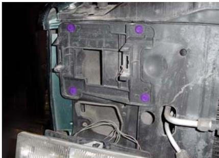
**4.** The next step involves removing the headlight units so they can be recessed approximately 1". To do this, remove the four factory bolts on each side holding the headlight assemblies to the radiator support. Unplug lights and remove assemblies from truck.
