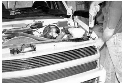
**5.** Pre-fit the Carriage Works Inc. shell & grille assembly to the truck by first attaching the two top tabs with the factory screws. With the vertical line of grille aligned with the edge of the fender, you can then drill holes in the exterior piece on fender. Close hood and check line.
