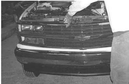
**1.** Remove the four screws attaching each parking light assembly to the grille. Remove the assemblies and unplug the lights from the back.
