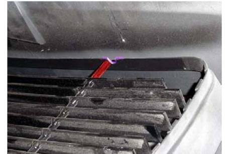
**STEP 1** Remove grille from truck by releasing clip. For protection tape off all painted or chrome surfaces on front. Lay grille face down on safe surface to work on.
