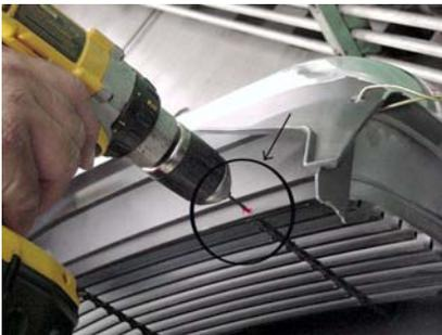
**STEP 4** Now insert Billet grille from front, leading in with the top. With clamps, hold back of billet grille flush with back of factory grille shell. Mark where center of rods touch grille shell. Remove Billet grille & drill 1/8" hole at the 3 marks just made.
