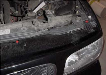
**STEP 1** Remove the factory grille shell by removing the (4) 7mm screws across the top of the shell.
