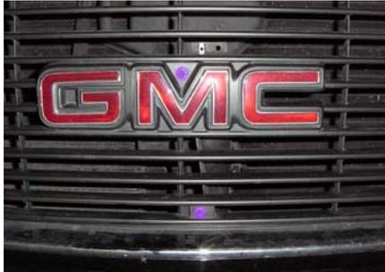
**STEP 2** Remove the (2) 7mm Screws holding the grille in the center of the GMC Logo, shown above in Purple.
