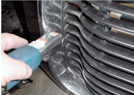
**STEP 5** Cut the vertical and horizontal bars from the center of the grille shell. Making sure not to remove the black ring remaining after cutting the bars.
