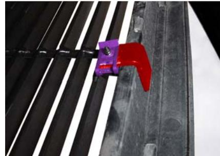
**STEP 8** Using the supplied brackets and hardware, install the brackets so that they hook under the bottom of the grille shell and tighten, as shown above. Re-install the grille shell.
