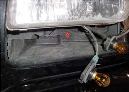
**STEP 4** Remove the 7mm Screw in the back of the parking light area of each parking light and the grille shell will be loose.
