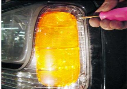
**STEP 3** Remove the (2) Phillips Head Screws from each parking lamp assembly and remove the lamp assembly.
