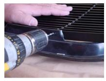
**Step 5** Center billet grille and mark locations where vertical rods meet the lip of factory shell. Drill 1/8" holes at each location. Fasten grille to factory shell with supplied hardware.
