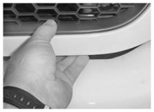
**STEP 2** Pull out on the 6-tabs located on the bottom of the grille shell.
