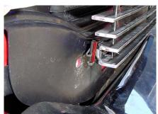
**STEP** 10 On models with no solid bar across the top,it may be neccessary to insert (1) of the provided spacers between the grille tab and the mounting tabs as shown for proper grille mounting.
