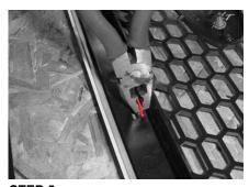
**STEP 5** Lay grille flat on a table with some protective covering so you don't scratch the front of your grille shell. Then using pliers, twist off tabs holding insert in place. Then grind tabs flush to shell surface.
