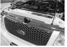
**STEP 1** Remove the 10 5.5mm screws from across the top of the core support and core support cover.
