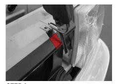
**STEP 3** Along top of core support you will find 2-notched areas closest to the headlights. You will need to notch the plastic with a hack saw or air-file as shown in picture.
