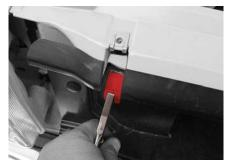
**STEP 4** After notching break the remaing plastic off using a pair of pliers. As shown in picture.
