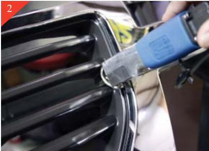
After grille shell is removed place shell face up on a protective surface, such as a blanket or rubber mat. Next you will be removing the center section of the factory grille shell, using a cut-off wheel or hack saw. Trim all vertical & horizontal plastic holding center in place.
