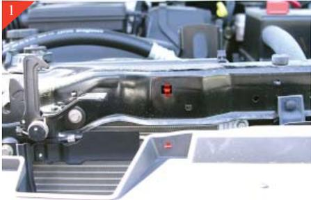
Remove the factory grille shell from vehicle, by releasing the (4) key hole tabs across the top of grille shell. Then there are (2) clips behind the parking lights on the driver & passenger side of grille shell, release by pulling straight out on shell. Then release (3) clips along the bottom of grille shell, by pulling straight out on shell.
