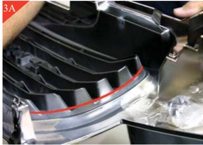
Lay grille shell face down, and using cut-off wheel or hack saw trim the remaining plastic. Using the Red Line as a guide for trimming (Fig 3A). Next sand edge smooth using a sanding block.
