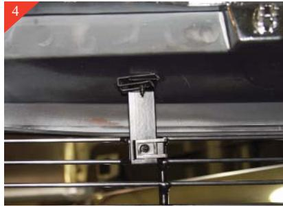
Next attach the Long "L" brackets to top of billet grille as shown. The long end attaches to billet grille with U-Clips and #8 x 5/8" Phil Pan head screw.
