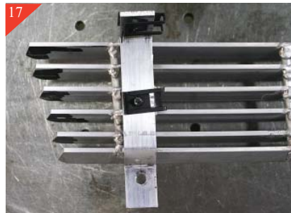
Next attach U-clips to the tops of the brackets only.
