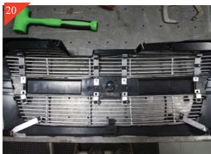
Then attach the (4) Brackets to the top of the billet grille using #8 x 5/8" black phil pan head screw. Then place the billet grille into the shell. Billet Grille must go into opening from the front. Next attach the bottom brackets to the billet grille using #8 x 5/8" black phil pan head screw. Pictured above is all brackets attached to billet grille and placed into opening.
