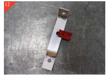
Next you will be attaching the brackets to the upper portion of the billet grille. All brackets used on upper portion of the billet grille are the same (pictured above). Do this by sliding a U-clip on to the center hole on brackets as shown above.
