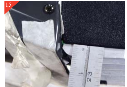
Showing a Reference measurement for the outer edge of the billet grille. There should be approximately 3/8" sticking out past the plastic shroud. After you get the depth correct you will need to clamp it in place.
