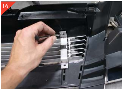
Next, mark locations of all holes for the top section of billet grille. Then drill a 3/32" hole in all marked locations.
