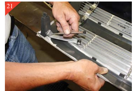
Next mark locations of all holes for the top brackets (Emblem Strip). NOTE: BEFORE MARKING THE BOTTOM HOLES YOU WILL NEED TO HOLD THE BILLET GRILLE FLUSH WITH FRONT OF OPENING AS SHOWN ABOVE.
