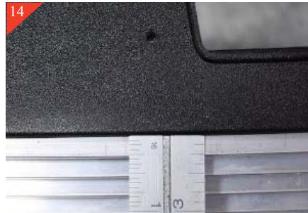
Lay grille shell face down and insert the Billet Grille from the back side and center into opening. Making sure plastic shroud is flat against top bar of grille. You should have approximately 1/4" (Measured from the center of billet grille.) of the billet grille sticking out past the top plastic shroud. As shown above.
