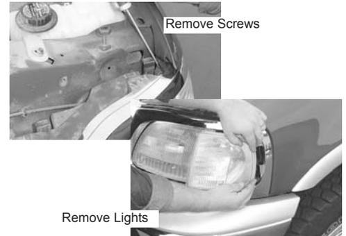
**STEP 3** Remove the parking lights by removing the torque screws as shown above. Then lightly pull the parking lights out.
