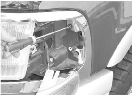
**STEP 4** Remove the 2 screws behind parking lights. The grille shell will be free at this point.
