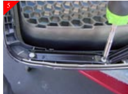
Remove the factory support brackets.
