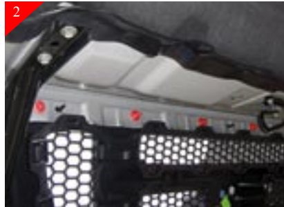
Remove the 6 (10mm) nuts holding the factory grille along the front edge of the hood shown above in red.
