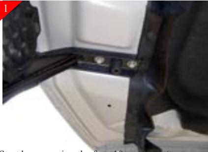
Start by removing the four 10mm bolts (two per side) that attach the grille frame to the hood.
