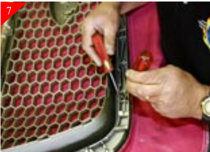
Once the tape has been removed, You carefully pry out the tabs that attach the honeycomb grille to the outer shell. There are 14 tabs to be released.
