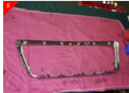
With the tabs released, the grille shell can now be removed from the honeycomb grille. Here is a picture of the frame without the honeycomb grille.
