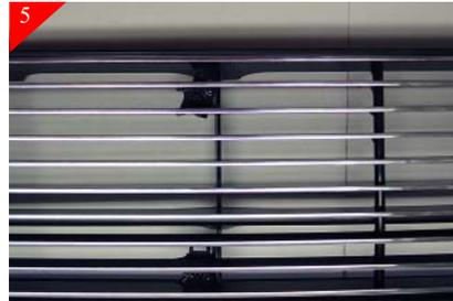
Center the Billet grille in the plastic shroud with the polished surface flush with the face of the shroud as shown.
