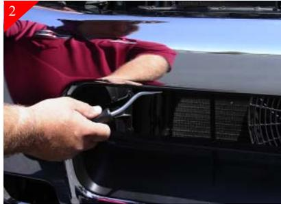
Next remove the (3) Plastic Push Rivets located along the top. Then remove the plastic insert.
