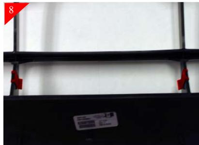
Place the U-Clips over the (4) holes just drilled as shown. Only the bottom 2 are shown above. Attach the grille assembly with the brackets to the plastic shroud with the supplied #8 screws. Next remove the (4) screws holding the billet grille to the brackets.
