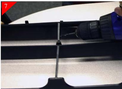
Next drill a 1/8" hole in each of the marked location in step 5.
