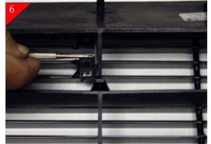
Mark the location of the (4) slots in the long leg of the brackets on the plastic shroud. Then remove billet grille from shell.
