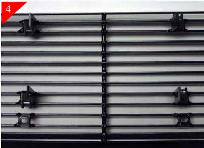
Attach the short leg of the brackets to the grille as shown using the #8 screws.
