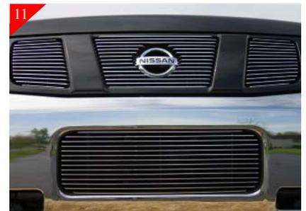
Re-install the plastic shroud into the bumper. Then Re-attach the grille to the brackets on the shroud.
