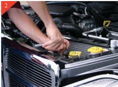
Next you will be removing the factory grille shell by removing (4) 13mm bolts along top of grille shell as shown.
