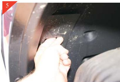
Then remove plastic covers found in wheel well as shown above. Using a flash light locate the 10mm nut and remove. Then in same area locate the white plastic tab, squeeze together to release and Headlight will be free. Then repeat process for the other side of vehicle.
