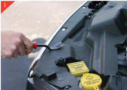
Open hood, then you need to remove plastic shroud covering core support, by removing or pulling up on the (8) plastic rivets as shown. Then tape under the Headlights using masking tape to protect paint surfaces when installing billet grille.
