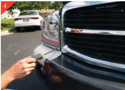
Next you will be removing the factory headlights. First remove the (2) (t-30) torx screws from front of the Headlight.
