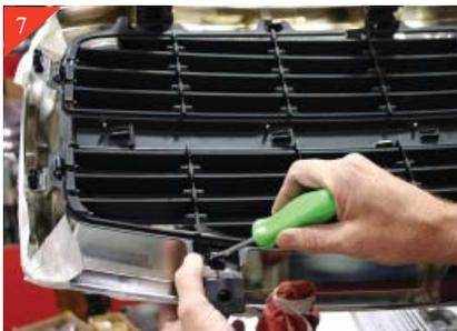
Lay grille shell face down on a protected surface so not to scratch during install. Remove plastic inserts by releasing tabs as shown (12) per side.
