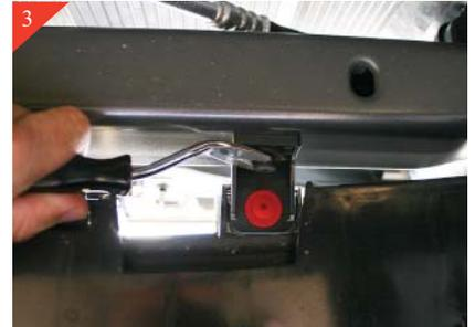
Next there are (4) plastic push pull rivets that are on the under side of the vehicle. You need to pull out on just the center portion of rivet to release. Picture above is shown from under vehicle.
