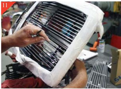
Then from the backside place the LONG bracket on bolts and then loosely attach bracket using 1/4-20 nuts as shown above. (Fig. 11-B showing bracket attached from the backside.) Repeat this same process using all long brackets to attach middle portion of billet grille.
