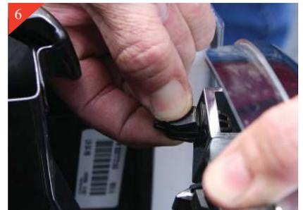
With the Headlights removed you can reach the remaining (4) black tabs holding the grille shell in place. Simply squeeze together to release. Remove grille shell from vehicle.
