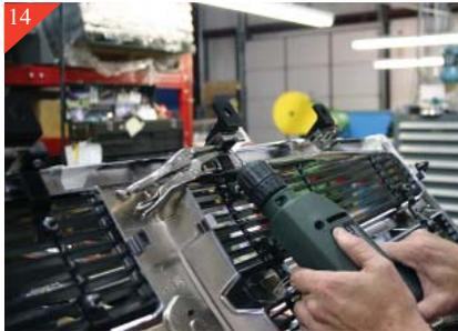
Then make sure billet grille is centered and flush with the face of the grille shell. Then using vice grips clamp all the loose brackets in place. Then using a 3/32" drill bit, drill holes in factory shell for mounting. Also you will need to drill for the center holes in the long brackets.
