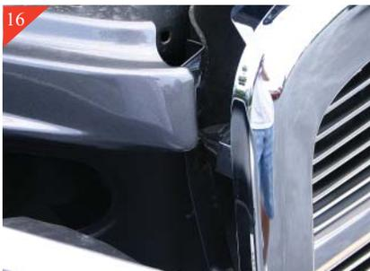
Next you will be re-attaching the grille shell back to the vehicle. Do so by simply lining up the black plastic tabs with holes and pushing in place. Then attach upper portion of grille shell using the factory 13mm bolts. Next push the plastic rivets in place from under vehicle (REF. Step 3). Then re-install the Headlights by pushing white plastic clip in place and then attaching the 10mm nut and also the 2 torx screws on front of headlights.
