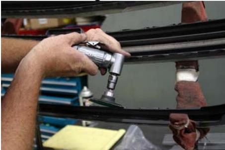
5. Next, use a fine grit sanding block to smooth all exposed surfaces. (For additional enhancement, paint the sanded surfaces to match the factory grille).
