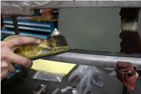
6. Using a file, remove the excess material in the corners around the emblem as shown.
