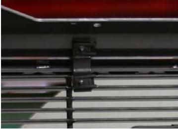
9. Attach the (4) hook brackets to the upper and lower sections of the grilles using the #8 screws and uclips making sure the hook brackets are secure on the grille bars.
