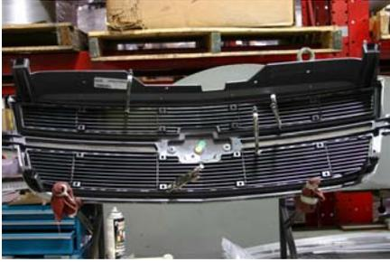
8. Attach the (4) Z- Brackets to the grille using the #8 screws and uclips as shown and drill a 1/8" hole thru the top of the bracket and the grille shell. Attach using the uclips and #8 screws.
