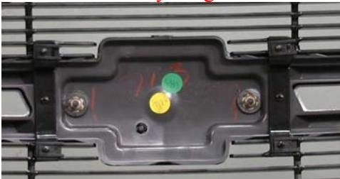
11. Attach the L-brackets to the lower grille section using (4) #8 screws and uclips. Drill a 1/8" hole thru the remaining hole in the bracket thru the bottom lip of the grill and attach using the #8 black screws and uclips.
