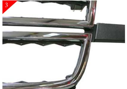
Pictured above is after cutting, sanding cut areas is optional. Do not remove material shown in "RED" in (Step 2).
