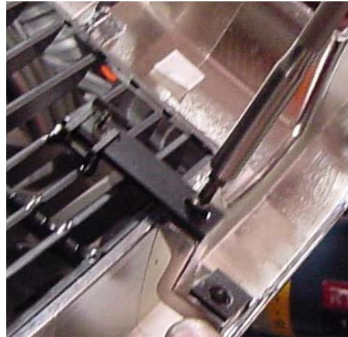
9. Attach the z-brackets to the top tabs on the upper grille inserts. Use a 3/32 drill bit to drill mounting holes into the grill shell at all of the bracket hole locations and secure with #8 screws. (Short bracket toward the center of the grille shell)
