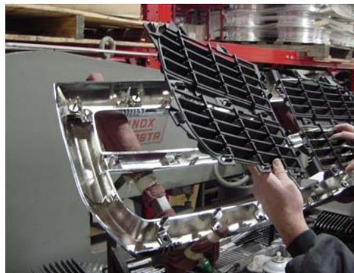
3. Remove the stock plastic insert from the back side. Use a flat blade screwdriver and twist the plastic tab away from the retainer as shown. There are 20 locations this needs to be done. Remove the stock insert.
