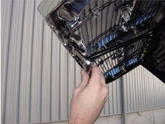
1. Remove (12) 8 mm nuts and bolts holding the shell onto the tube frame
