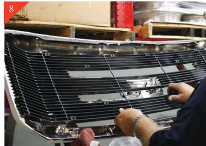
Place the billet grille into the open and center. Next you will be attaching all the brackets to the billet grille.
