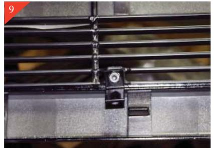
Loosely attach the ( L ) shaped brackets to the bottom of billet grille, with the short side of bracket attaching to billet grille as shown above.
