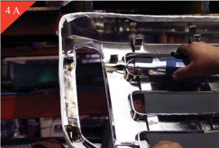
Next using a cut-off wheel or a hack saw it will be necessary to remove some of the tabs (Fig 4A). The next step (Fig. 4B) shows the tabs that need to be removed.
