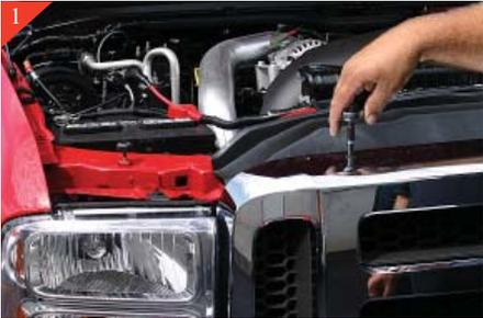
Open hood and remove the (4) 7/32" bolts holding stock grille shell in place. Then remove rubber core support cover by pulling up on the plastic rivets.
