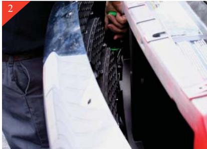
Next pull the stock shell slightly forward, and reaching behind the stock shell release the (5) clips at the bottom of the stock grille shell. If needed use a flat blade screwdriver to aid in releasing the clips as shown above.
