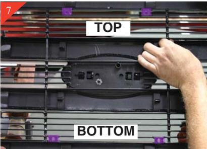
Take note before placing the billet grille into opening. The Top (2) "Center Tabs" are spaced out more from the vertical rods than the bottom (2) as shown above.
