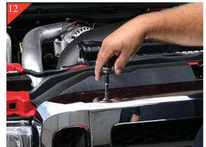
Place the shell back on vehicle and align. Then replace the stock 7/32" bolts that attach across the top of shell.
