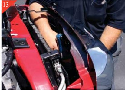
Now you will need to drill a hole in the fiberglass framing to allow the bottom "L" brackets to attach to vehicle. Reach behind the grille shell and locate the bottom "L" brackets. Then drill a 3/32" hole in each. Then attach using #8 x 5/8" screw in just drilled location.
