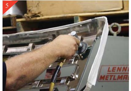
After the tabs have been removed, you will need to sand or grind all the cut areas smooth with shell.
