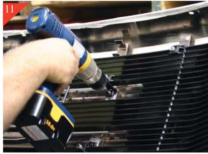
Making sure (Z) brackets & (U) Clips are aligned with each other. Drill a hole using a 3/32" bit down thru bracket and U clip. Then attach using a #8 x 5/8" Phil pan screw. Repeat this process for all (Z) brackets. Billet grille will be attached to stock shell at this point.
