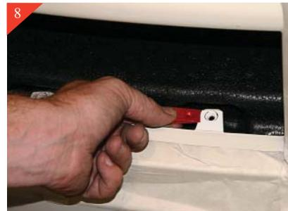
8 Next attach the supplied L-brackets to the factory mounting tabs in the lower portion of the grille shell. By placing U-clips on the factory tabs then attaching the L-brackets to the clips using #8 x 5/8" screws.
