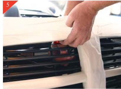
5 Pull up on factory grille and release (2) upper tabs from slots and remove factory inserts. One of the tabs is shown above in Red.
