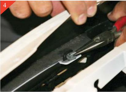
4 Squeeze the (2) Metal Clips in the Top horizontal bar holding each grille insert in place to release.
