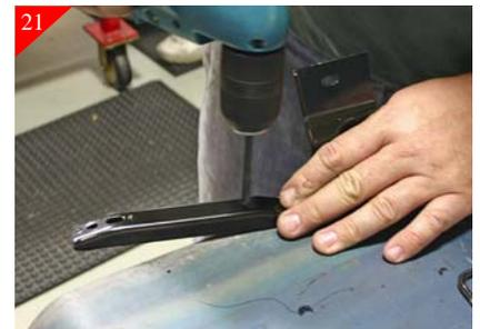
Next starting with the metal top portion drill a 1/4" hole in the just marked locations (Ref. Step 20) as shown above.
