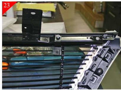
Then attach the supplied top bracket using 1/4-20 nut and 1/4-20 nyloc nut as shown above. Then place billet grille into opening and center. Then re-install the top metal portion using stock torx (t-20) screws (Ref. Step 3) you will also need to place the supplied square tab on the middle (2) torx hole locations. Next attach billet grille to top brackets using #8 x 5/8" Phil head screws.
