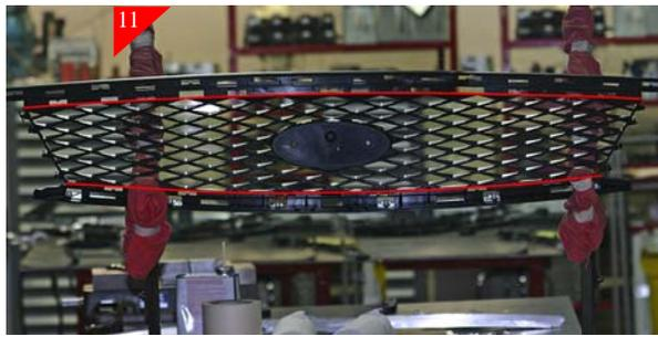
Next you will be cutting the "egg crate" section of the plastic center. Using a cut-off wheel or hack saw cut along the RED line shown above. You need to keep the top & bottom portion of plastic center.
