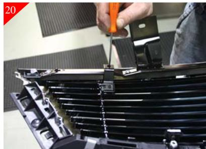
Then using a scribe mark the locations of the holes as shown above. Then remove the brackets that are attached to the billet grille. Also remove the billet grille and remove the top metal portion and the bottom plastic portions of stock grille.
