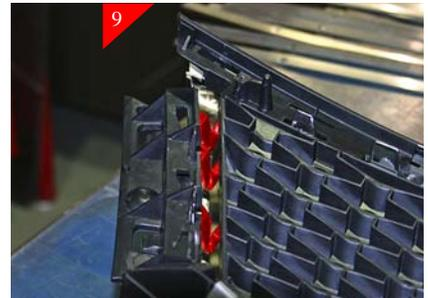
Next using a air file or a hack saw cut as shown above. Leaving the pieces attached to grille shell as shown.
