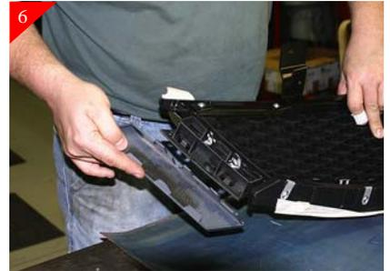
Remove Plastic covers from the drivers & passengers side of grille shell by unclipping, as shown above.
