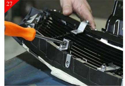
Then re-install the bottom plastic portion as shown using #8 x 5/8" Phil Pan head screws. Then attach all bracket to billet grille using #8 x 5/8" Phil pan head screws. After all bracket are tight and secure re-install the stock shell back to the vehicle (Ref. Steps 1-4).
