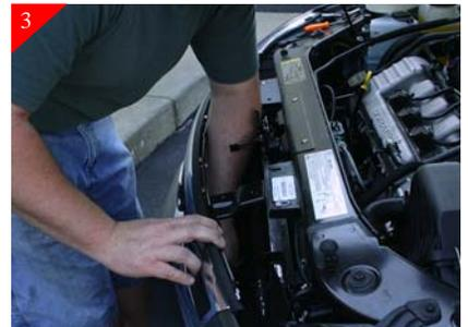
Remove (6) 8mm bolts from the bottom of the stock grille shell by reaching behind stock shell as shown above.
