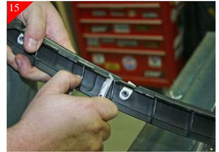
Using a utility knife notch plastic where it meets the bracket (Ref. Step 13).
