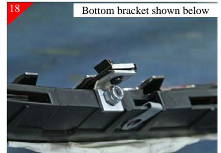
Place billet grille into opening and center. Then re-install the top metal portion using stock torx (t-20) screws (Ref. Step 3). Next you will be attaching the bottom plastic portion to chrome shell. Attach u-clip to bracket (Ref. Step 13) for location as shown above.
