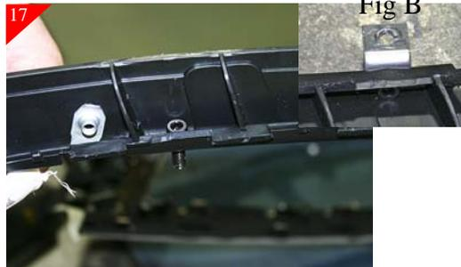
Then place the supplied 1/4-20 bolt as shown. Then attach the bracket with Nyloc 1/4-20 nut (Fig B).
