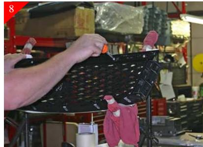
Remove the (6) Torx (T-20) along top of grille shell as shown. After screws are removed top portion will be free.
