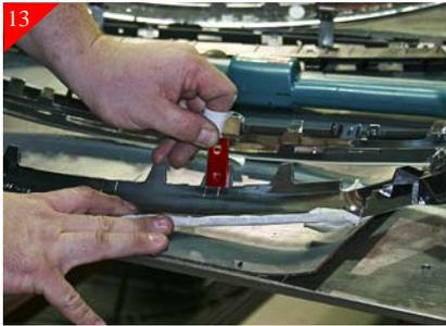
Next using the supplied Tab shown above. Place them on the 2nd tab from the left and the right side of chrome shell as shown. Then using a scribe mark the locations of the holes. Then using a 3/16" drill bit drill the just marked locations.
