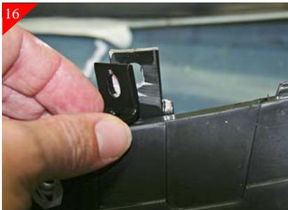
Next align the supplied bracket with previously installed bracket as shown above. Then using a scribe mark the location of the hole in the plastic. Then using a 1/4" drill bit drill in marked locations.
