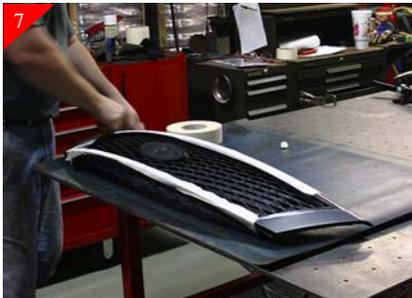
Next tape stock grille shell using masking tape to protect during install.
