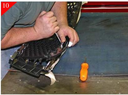
Next release the tabs that is holding the plastic center. It maybe necessary to use a regular screwdriver to aid in releasing the tabs.
