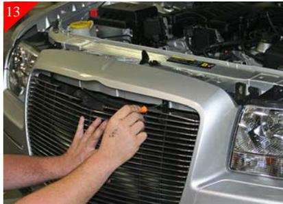
Place Billet Grille into opening and center. Using a scribe mark where the TOP brackets meet the vehicle as shown. Then remove billet grille and drill 1/4" hole in each of the marked locations.
