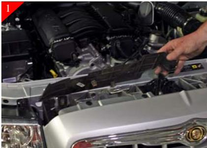
Open hood and remove the plastic shroud by un-snapping clips as shown above.
