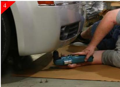
Next you will need to remove the (10) 7mm bolts that are under the front end as shown. This helps to loosen the front end for the next steps.
