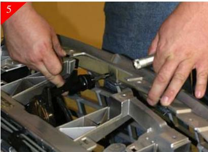
Next remove (6) #2 square drive screws from backside of the stock grille shell. There are (4) across the top, (2) on opposite sides. With screws removed next slightly pull out on grille shell to unsnap. You may want to use a screwdriver to aid in the release of the clips.
