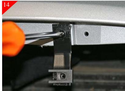
Remove the brackets from the backside of the billet grille. Then place u-clip on the just drilled holes from STEP 13. Then attach the brackets to the just placed u-clips as shown.
