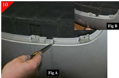
In the grille shell opening you will need to trim the plastic shown above (Fig. A) using a utility knife. (Fig. B) shows plastic trimmed away.
