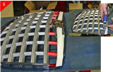
Next you will be removing the top portion of the stock grille shell that contains the chrysler emblem. Do so by cutting the vertical supports shown above in RED. Make sure to leave extra material (On the Emblem Side.) So that you can come back and do finish sanding.
