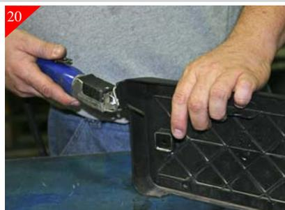
You will also have to trim the sides in order for the contour to fit correctly. Start with trimming a small amount away and hold the frame up to vehicle to check fitments then trim the necessary areas in order to fit. You will need to file all the cut areas smooth for appearance. Then attach using stock hardware.
