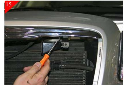
Next hold the stock trim piece (Chrysler Emblem) up to the vehicle and center. Then using a sharpie mark where the brackets hit.
