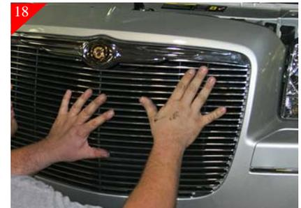
Place billet grille into opening and center. Then attach to the top brackets using supplied #8 x 5/8" Phillips head screws. Then use the supplied #8 x 1" to attach the bottom .
