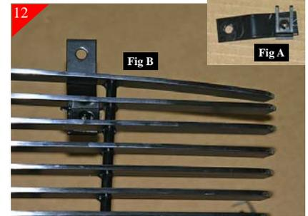
Then place U-clips on brackets as shown above (Fig A). Then attach brackets to billet grille (Fig. B).
