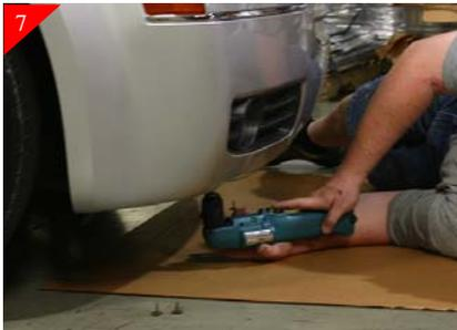
After the center section is removed. You can re-install the (10) 7mm bolts that were removed in step 4.
