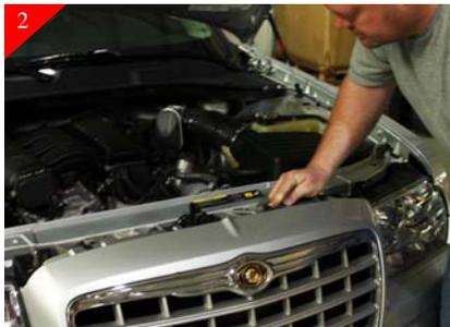
Next remove the (4) plastic push pull rivets that are across the top of the shell as shown.
