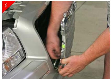
There are also (4) #2 square drive screws that are along the bottom. **NOTE: You may want to use a #2 bit and an open end wrench to aid in the removal of the screws.**
