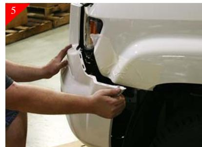
Then slightly pull outward on the front end as shown to release. The front end will un-snap at this point, but will still be attached by the (2) center bolts on the bottom front.
