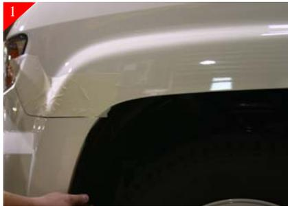
Tape both driver & passenger sides of front fenders as shown using masking tape to protect during install.
