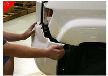
After paint has dried remove cardboard and snap the front end back to vehicle and attach using the 10mm bolts.
