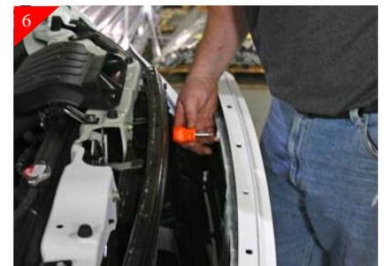
When the front end is loose slightly lean the front end forward and remove (9) phillips screws holding center section of stock grille shell as shown. You may want to use a "Stubby or Short Screwdriver."
