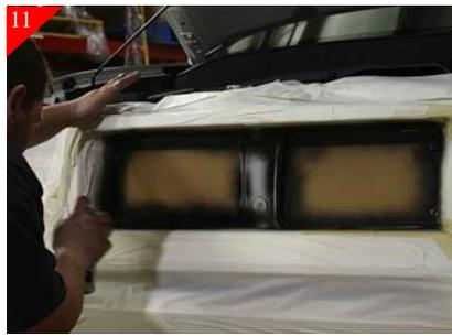
Wipe off area to be painted using a damp cloth.. Then using Flat Black paint center section as shown. Let paint fully dry then a second coat maybe necessary. Remove 1 screw at a time and quickly paint where screw was while holding cardboard. You also will want to hold the backside of cardboard during painting of the screw holes.
