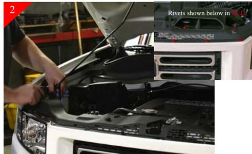
Next open hood and remove the (9) Plastic push-pull rivets along plastic shroud that cover core support. Then remove the (3) plastic push-pull rivets holding air induction as shown. Plastic shroud will be free at this point.
