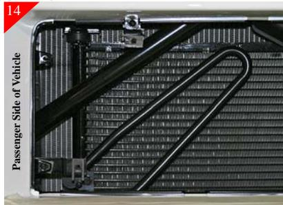
Attach the bottom bracket as shown long end of the bracket to the truck. Attach the top bracket as shown.
