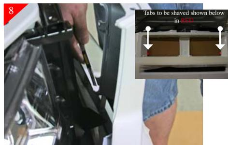
With center section removed, you will need to shave off the raised section of the BACKSIDE of the bottom (2) tabs. Lean the grille shell forward and then using a utility knife shave off the raised sections as shown above.
