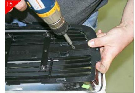
Next you will be reinforcing the backside of the shell. Using the supplied braces, one per side of shell. Butt the brace against the brackets the are holding the billet grille in place. Then attach the brace by using a #8 x 5/8" Phillips head screw and U-clip.
