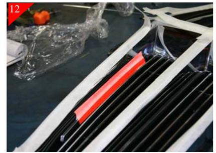
Next place the billet grille into the correct openings. Then to help hold the billet grille in place during install, tape the First and Last bar to the chrome shell. Shown above in RED.
