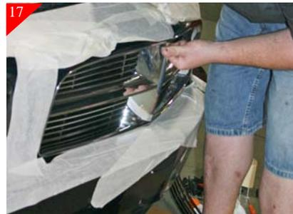
Next attach stock shell back to vehicle. First go ahead and put the factory air deflectors back in place and attach with the factory plastic rivets, also attach the wiring harness. Then place the shell back on vehicle and push slighty until it snaps in place. Then attach shell using factory screws (Reference step 5.). You will need to install the lower billet grille before attaching the factory plastic shroud (Ref. step 3).
