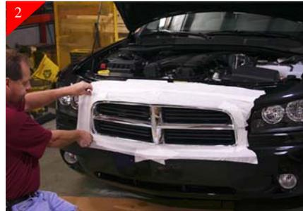
Using masking tape, tape off the front end of the car as shown to protect during install.
