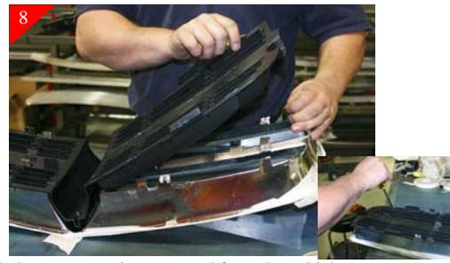
With the center section removed from the vehicle. Tape the face of the shell using masking tape to protect during install. Then lay shell face down on a work surface and release the clips as shown above. There are (8) Clips total per side. Start with the outside ones first then release the center ones.
