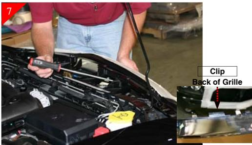
Next release (4) the clips holding the center section of grille shell. It may be necessary to use a large screwdriver or pry bar to aid in the release of the clips. There are 2 clips along the top of the center portion of the grille and there are 2 along the bottom.
