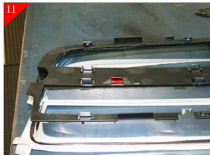
Next lay chrome shell face down. Then on the drivers side of the shell you will need to trim the above tab (Shown in RED.) and sand smooth. After trimming put the black plastic back in place.
