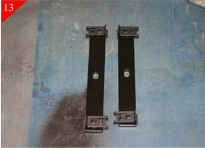
Next place the supplied U-clips on both ends of the brackets as shown. NOTE: 1 long and 1 short per side of vehicle.
