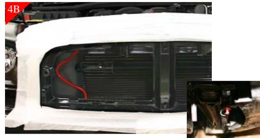
Continuing with the removal of the air deflectors. On the passenger side you will need to un-clip the wiring harness from the deflector shown above in RED. Then reaching under vehicle remove the 2 rivets holding the bottom of the air deflectors.
