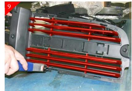
Next you will cut out the vertical bars using a hack saw or cut off wheel (Shown In RED). Then using a utility knife and or a sanding block, smooth up or blend all the cut areas. See next step for reference.
