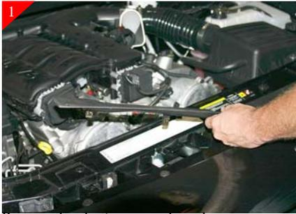
Remove the plastic covers along the core support by pulling slightly upward to release.
