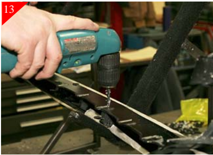
13 Using a 3/16" drill bit, drill in the just marked locations as shown above.
