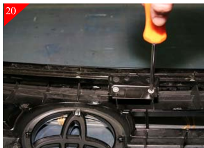
20 Going back the stock center portion of the grille shell that you removed. Remove the stock hood release bracket as shown.
