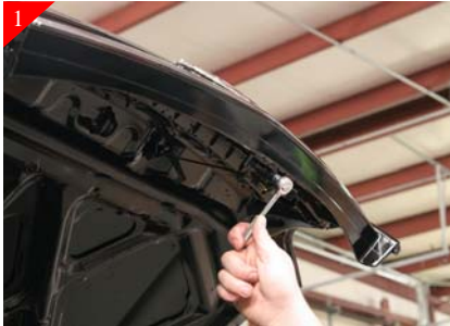
1 Open hood and remove (2) 10mm. Bolts that hold stock hood release.
