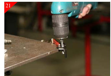
21 Drill the mounting holes in the stock hood release bracket using a 9/32" drill bit as shown above. Caution please use a pair of vice grips or other clamp to hold during drilling.
