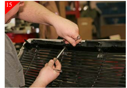
15 Attach billet grille to the just place brackets and attach using 1/4-20 x 3/4" bolts and 1/4-20 nuts. It will be necessary to use a open end wrench to tighten bolts.
