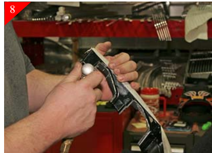
8 Next you will be sanding the sides of the grille shell flush using a sanding block or air sander.
