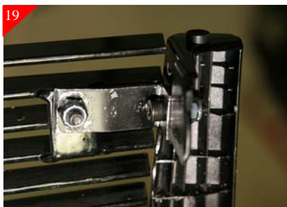
19 Attach brackets to the just drilled area using the supplied 1/4-20 x 3/4" bolts and 1/4-20 Nyloc nuts.
