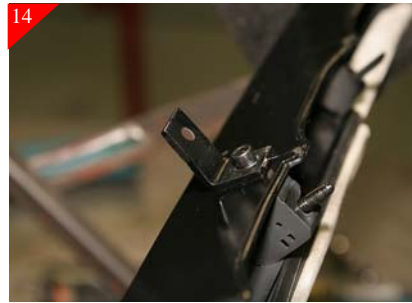
14 Attach bracket to stock shell in the just drilled location using 1/4-20 x 3/4" bolts and 1/4-20 Nyloc nuts as shown above.
