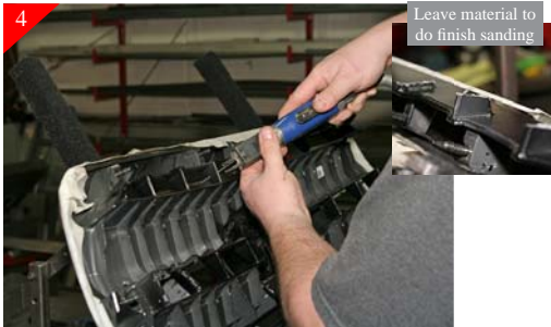
4 Next you will be removing the center portion of the stock shell using an air saw or hack saw. Making sure to leave material so you can come back and do finish trimming and sanding. Trim the top portion of the grille shell as shown above, again leave material to sand to.
