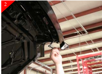
2 Remove (6) 10mm bolts that surround the stock grille shell. Grille shell will be free at this point.
