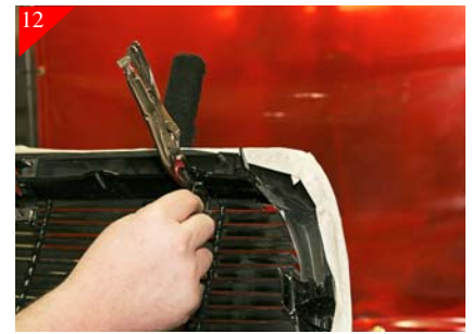
12 Using a scribe mark the hole locations in brackets where they meet the out stock shell as shown above. After marking holes remove the billet grille from opening.
