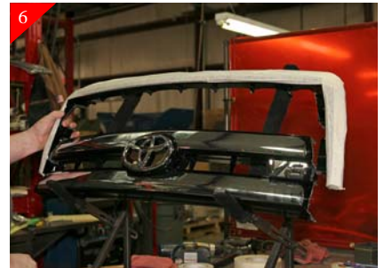
6 Shown above is after cutting the center portion of the stock shell out.
