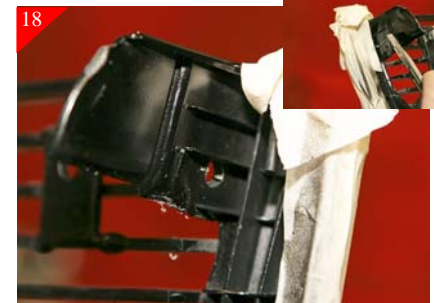
18 Trim the plastic ribs using a utility knife that are on the opposite side where top brackets attach, so that the nut will lay flat against shell.
