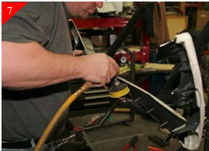
7 Start with sanding the top of the stock shell cut areas smooth with the stock shell as shown above taking care during sanding so as not to scuff the stock shell.
