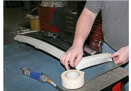
3 With grille shell removed go ahead and tape the face of the grille shell using masking tape so that no damage occurs during install.
