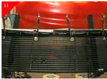
11 Place billet grille into opening upside down for the time being as shown above. Then using some vice grips clamp in place. Also check alignment on the face of the grille to make sure that you are flush.
