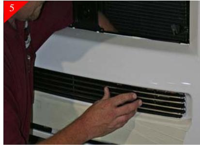
Place the center bumper billet grille into opening and center. Reach thru the upper grille opening and mark the holes for the brackets to attach bumper grille as shown. Then remove billet grille from opening and also remove the brackets from the billet grille.
