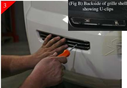
Slightly lean the grille shell forward, then hold U-Clip on the backside of the grille shell and attach using the supplied #8 x 1" phillips head screw. (Fig. B shows Backside to show attachment of the U-Clips). Note: you may want to use a pair of pliers to hold.
