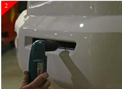
Then drill holes in just marked locations using a 1/4" drill as shown.
