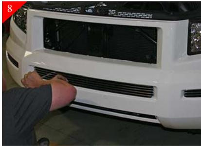
Now place the billet grille into opening and center and attach using #8 x 5/8" phillips head screws.
