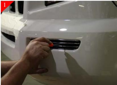
With steps 1 Thru 8 completed. Next Place the small outer billet grille into the opening and center. They are left and right specific. With grille centered mark holes with scribe as shown and remove.
