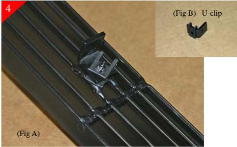
Next attach the supplied U-clips on the slotted side of the "L" brackets only (Fig. B). Then attach the brackets to the billet grill using the supplied #8 x 5/8" as shown (Fig A.).
