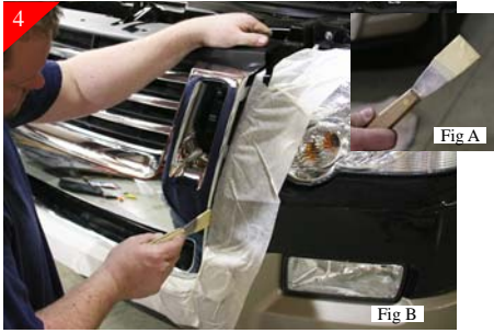
Using a taped up putty knife to aid in the removal of stock grille shell (Fig A). Slide the putty knife in between stock shell (chrome) and the front end (painted) and slightly pull out to release the clips holding shell in place (Fig B). There are 12 clips surrounding shell. Shell will be free at this point .
