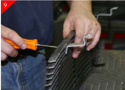
Attach the Top brackets to billet grille using the supplied #8 x 5/8" Phil pan head screws as shown above.
