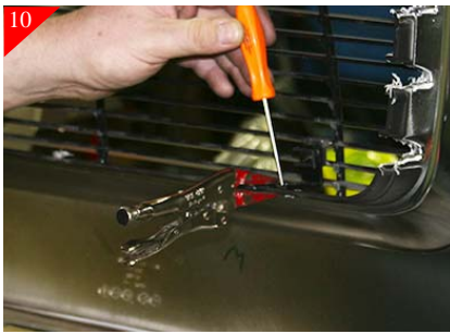
10 Place billet grille into opening and center. Using a pair of vice grips clamp the bottom brackets flush with the backside of the grille shell as shown.
