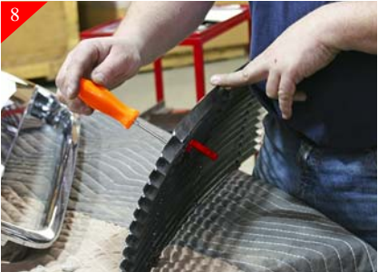
Attach the bottom brackets to billet grille using the supplied #8 x 5/8" Phil pan head screws as shown above.
