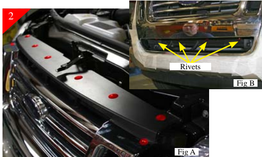
Remove (8) plastic phil head screw from along the top of stock grille shell as shown(Fig A). Then located in the bumper opening remove (4) plastic rivets (Fig B).
