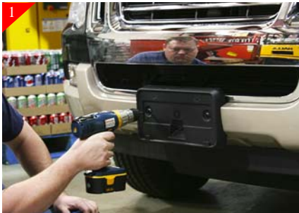
Open hood and remove license frame holder by drilling out the (3) Aluminum Rivets. Using a 5/16" drill to remove.
