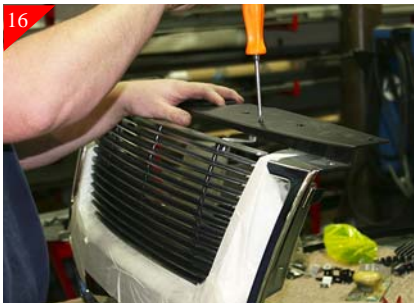
16 Place billet grille back in stock opening and center. Attach the top portion of the billet grille with the supplied #8 x 5/8" Phil pan head screws as shown above.
