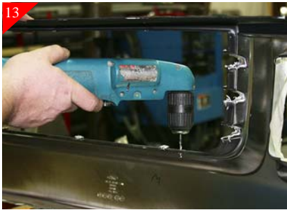
13 After marking holes remove the billet grille from opeing. Using a 3/16" drill bit drill in the just marked locations.
