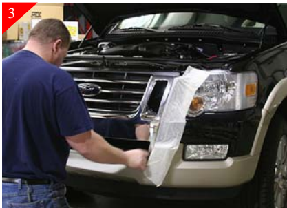
Using masking tape, tape the front end of vehicle to protect during installation.
