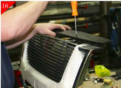
Place billet grille back in opening and center. Attach the top portion of the billet grille with the supplied #8 x 5/8" Phil pan head screws as shown above.
