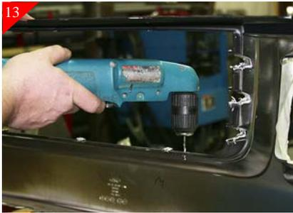
After marking holes remove the billet grille from opening. Using a 3/16" drill bit drill in the just marked locations.
