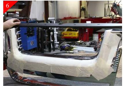
After center section is removed you will need to sand all cut areas smooth using a sanding block.
