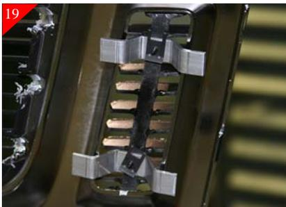
Place the Wing grille into opening and center. Then attach using the supplied Wing brackets and #8 x 5/8" phil pan head screws as shown above. Top of Wing grille uses Shallow bracket and the bottom of Wing grille uses Deep bracket.
