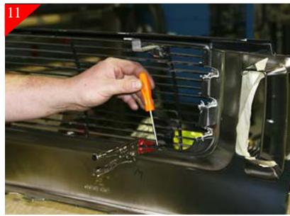
Using a scribe mark the location of the holes in the bottom bracket as shown.
