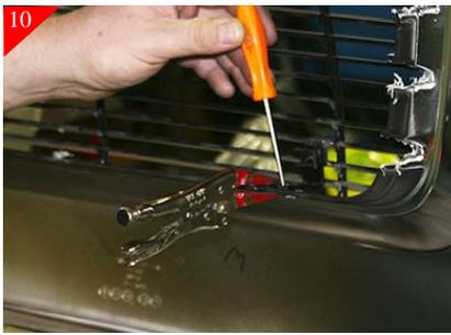
Place billet grille into opening and center. Using a pair of vice grips clamp the bottom brackets flush with the backside of the grille shell as shown.
