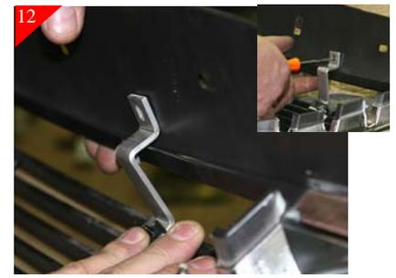
Then hold the top bracket against grill shell as shown and mark the loations of the holes in the top brackets.
