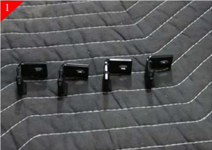
Place supplied U-Clips on all the SHORT ends of the supplied bumper "L" brackets as shown above.
