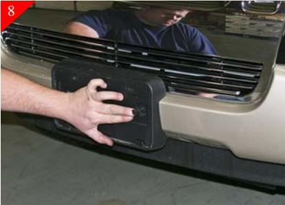
If your state requires you to have a front license plate. Re-install the license plate holder using the supplied push pull rivets as shown above.
