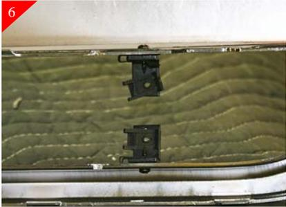
Using a 3/16" drill bit, drill in the just marked locations. Attach the brackets using the supplied U-clips and #8 x 5/8" Phil pan head screw as shown above.
