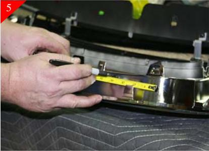
It will be necessary to measure and remark hole locations so that you will be able to reach for drilling of the holes. Measure and mark on the outside of the opening. You will not be able to fit a drill on the inside of the opening.
