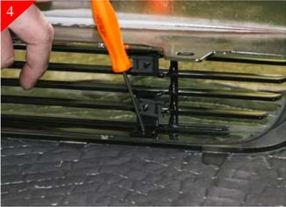
Mark the locations for holes in brackets as shown above. Then remove the billet grille from opening also go ahead and remove the bracket from the billet grille.
