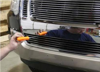
Place stock shell back on vehicle and snap clips in place. Replace the (4) plastic rivets in bumper opening. Replace the (8) plastic Phillips head screws across the top of the shell. Place the billet grille into opening and center, attach using the supplied #8 x 5/8" Phil pan head screws
