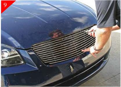
Attach the billet grille to the brackets using #8 x 5/8" Phil pan head screws. Carefully close the hood and check for alignment of the hood line. You may need to adjust a little, do so by loosening the #8 screws and adjust accordingly and then tighten.
