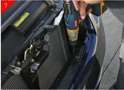
Remove the billet grille from the opening and using a 3/16" drill bit, drill in the just marked locations as shown above.
