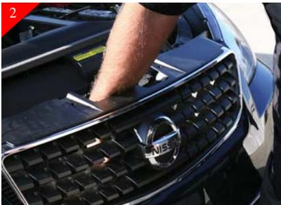
There are (4) clips that are located at the bottom of the stock grille shell that need to be released. Do so by reaching behind the stock shell and pulling up on the clips to release. Shell will be free at this point.
