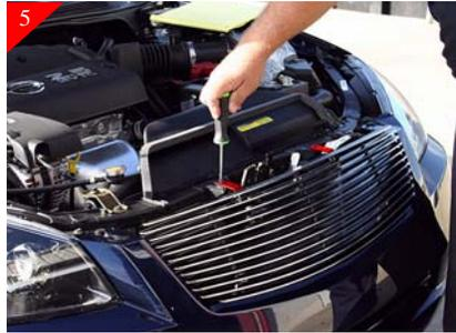
Place billet grille into opening and center. Then attach the top of the billet grille as shown above using the supplied #8 x 5/8" Phil pan head screws.
