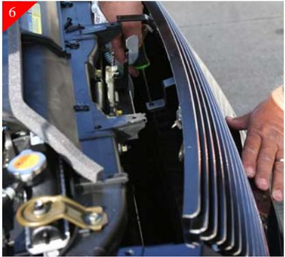
Next you will be marking the holes for the lower brackets. Do so by reaching behind the billet grille and mark the hole location in the bumper support. If necessary but not recommended in order to reach the lower brackets you may have to undo the top portion of the billet grille, but make sure that the billet grille is flush with the opening before marking.
