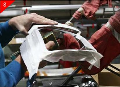
Using a sanding block sand all the cut areas smooth with shell.
