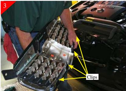
Located along the bottom of the stock grille shell there are (4) clips that need to be released, do so by squeezing or pulling up on them. Grille shell will be free at this point.
