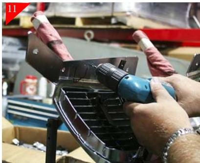
Loosen the bracket so you can swing them down out of the way for drilling. Using a 3/16" drill bit, drill in the just marked locations as shown above. After drilling place a supplied U-clip on all the top brackets and then attach using #8 x 5/8" Phil pan head screws.
