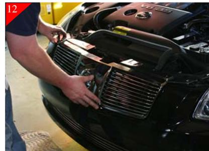
After tightening all brackets simply re-install the grille shell back on vehicle by pushing in on the bottom portion of shell to snap the clips back in place and re-install all the rivets along top of the grille shell (Ref. Steps 1-3).
