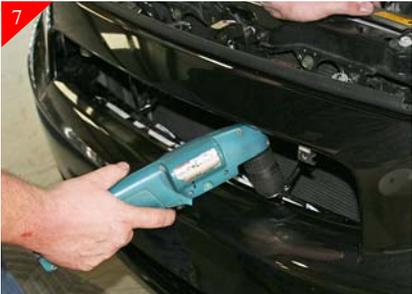
After marking holes remove the billet grille. Then using a 3/16" drill bit, drill in the just marked locations.
