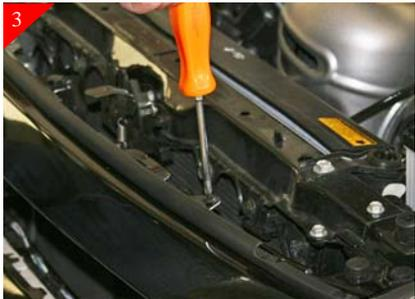
Remove the (2) plastic push pull rivets that are along the top of the stock grille shell as shown above.
