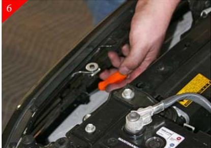
Then place billet grille into opening and center. Then attach the billet grille to the top brackets. Then mark the location of the hole in the lower bracket as shown above. Make sure to align the bottom portion of the billet grille before marking hole locations.
