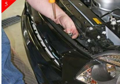
Attach the top brackets using the supplied #8 x 5/8" Phil pan head screws and washer in the just removed rivet location (Ref Step 9).
