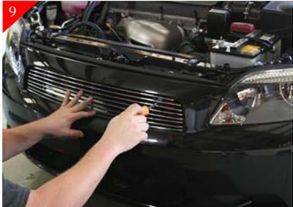
Place billet grille back into opening and center. Then attach billet grille to the brackets using the supplied #8 x 5/8" Phil pan head screws.
