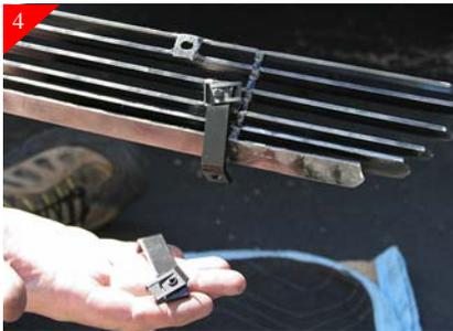
Next place a u-clip on the "long" or straight end of the supplied bottom brackets as shown. Then using #8 x 5/8" Phil pan head screw, loosely attach the brackets to billet grille as shown.
