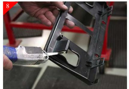
Next using an air saw or hack saw cut the top tabs off shown above. Snap the bottom tabs of the license frame holder in place and center. Mark the location of the slotted tab on the backside of the holder and remove holder. Drill a 3/16" hole in the just marked location. Then snap the license frame holder back in place and attach to bracket on front of billet grille (Ref. Step 3) using the supplied washer, 10-24 x 2", and 10-24 Nyloc nut.
