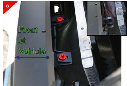
Next you will be attaching the top bracket to the factory 8mm screws shown above. (Please Ref next step for diagram of attachment of brackets).
