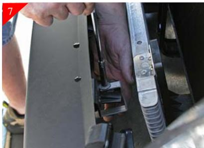
Next place the billet grille into opening and center and then rotate the bottom brackets around so they catch the bottom of opening. Then attach the billet grille to top bracket using the supplied #8 x 5/8" Phil pan head screw and tighten.
