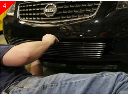
4 Place billet grille into opening and center. Reaching up thru from the bottom "splash guard area", rotate the brackets around so that they catch the middle plastic in stock bumper opening.
