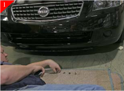
1 Remove the (5) 10mm bolts from under splash guard, located under front end of vehicle.
