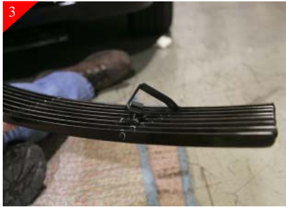
3 Loosely attach the brackets to the billet grille as shown above using the supplied #8 x 5/8" Phil pan head screws.
