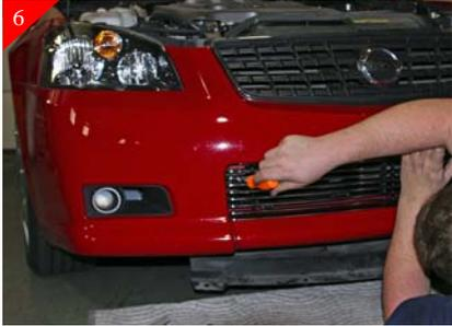
6 Place billet grille into opening and center, then attach billet grille to the brackets using the supplied #8 x 1" Phil pan head screws. Tighten the bottom brackets without overtightening. Re-attach the plastic shroud (Ref. Step 1) using the stock plastic rivets. Bumper installation is complete.
