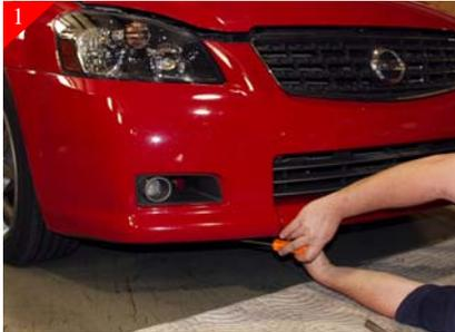
1 Located under the front end of the vehicle remove the (5) plastic rivets that hold plastic shroud in place, just let plastic shroud hang down.
