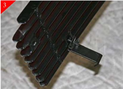
3 Place the supplied U-clips on the bottom brackets, u-clips attach to the side with hole. Then loosely attach the bracket to the billet grille using the supplied #8 x 1" Phil pan head screw as shown above.
