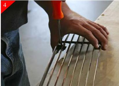
Loosely attach the brackets to the lower billet grille using the supplied #8 x 5/8" Phil pan head screw. (Ref. step 3) for the placement of the brackets. Then place the billet grille into opening and center.
