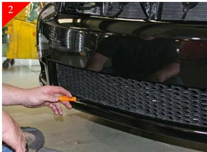
Remove the bottom "egg crate" portion of stock grille by releasing the clips that surround, just as in removing the upper portion (Ref. step1).
