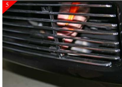
Reaching thru the upper opening you will need to mark the location of the hole in the bottom bracket as shown above. Check to make sure the billet grille is flush with opening, also check that the bottom bracket is flush with the backside of the lip in bumper opening. After marking remove the billet grille.
