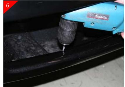
Using a 3/16" drill bit, drill in the just marked location in the bumper opening as shown above. Then place a supplied u-clip on each of the just drilled holes. Then remove the bottom brackets from the billet grille, and attach them using the supplied #8 x 5/8" Phil pan head screw to the just placed u-clips in bumper opening.
