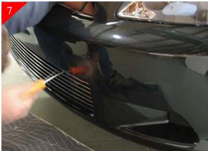
Place billet grille back into opening and center. Rotate the upper brackets so that they catch the top portion of the bumper opening. Then attach the bottom portion of the billet grille using the supplied #8 x 5/8" Phil pan head screws.
