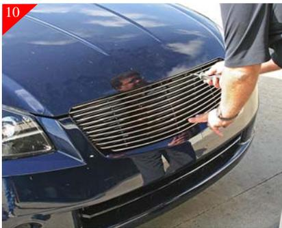
Attach the billet grille to the brackets using #8 x 5/8" Phil pan head screws. Carefully close the hood and check for alignment of the hood line. You may need to adjust a little, do so by loosening the #8 screws and adjust accordingly and then tighten.
