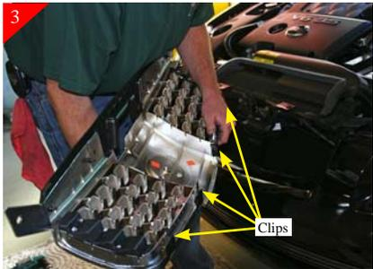
Located along the bottom of the stock grille shell there are (4) clips that need to be released, do so by squeezing or pulling up on them. Grille shell will be free at this point. You will not be using the stock grille shell for the rest of the install.
