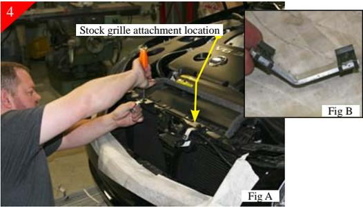
Place the supplied U-clips on the Upper Brackets as shown above (Fig B). Attach them in the stock grille attachment locations, the long end of the bracket attaches to the vehicle using the supplied #8 x 1" Phil pan head screws & washers.
