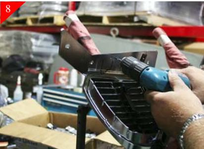
Remove the billet grille from the opening and using a 3/16" drill bit, drill in the just marked locations as shown above. After drilling remove the lower brackets from the billet grille.
