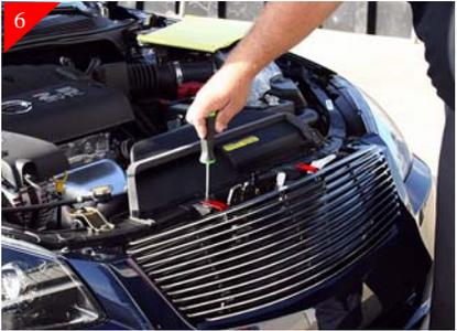
Place billet grille into opening and center. Attach the top portion of the billet grille to the top brackets using the supplied #8 x 5/8" Phil pan head screws.
