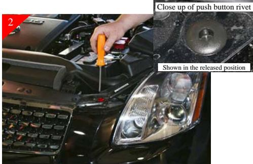
Then remove (2) plastic rivets on grille shell shown above in "RED" by pushing in on the inner portion of the rivet to release. Then pry up to remove.
