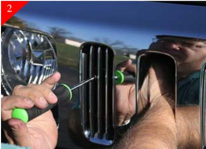
Place billet grille into opening and center, while reaching thru the opening next to the one you are working on, turn the "Flat" bracket sideways and tighten while holding in place. Repeat for remaining openings.
