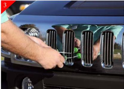
When you get to the last one, you will need to use (2) screwdriver to aid in the installation of the last billet grille. One to hold the bracket and one to tighten up the grille.
