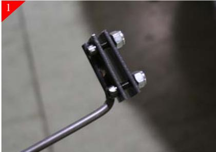
**(Fig. A)** First set up your new hood release bracket as shown above. Then slip the new release over the stock hood release so that the new release sandwiches the stock one and tighten. The new hood release is accessible from underneath the chome shell. **(Fig. B)** Next Place the supplied bolts thru the mounting tab in billet grille. Place a flat bracket on the backside of the billet grille with the bolt going thru the bracket. Then thread the toggle assembly onto bolts as shown above.
