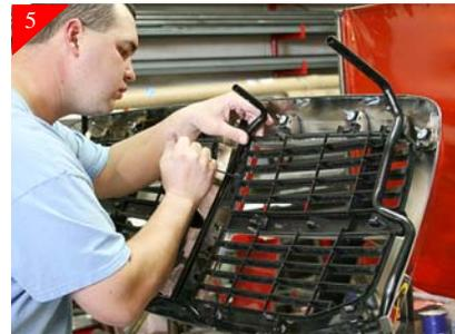
Lay the stock shell face down on a protective work surface. Locate and release stock clips holding center portion of the stock shell, there are (11) per side. You may use a regular screwdriver to aid in the release of the clips. Centers will be free at this point.
