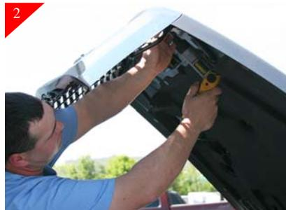
Remove (6) 8mm nuts and (6) 8mm bolts that surround and hold stock grille shell to vehicle.
