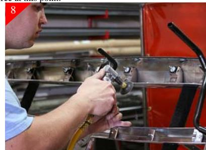
With all the clips removed using a sanding block or air sander sand all cut areas smooth as shown.
