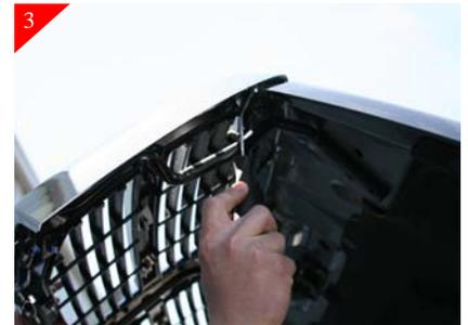
The Stock grille shell has a rubber weather strip across the top of the shell. To release use a large regular screwdriver to pry out while being careful as to not cause any damage. Do to the heat from the sun the strip can be sticky.
