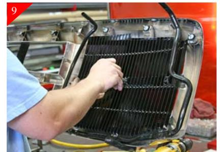
Center billet grille into opening making sure to have the same amount of gap on the left and right of the billet grille. Then using a scribe mark the hole locations where they meet the stock shell as shown above.
