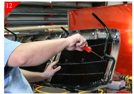
Attach billet grille to the just place U-clips using the supplied #10 x 1 1/2" Phillips head screws. Small adjustments can be made by loosening the Phillips head screws move a necessary and then tighten.
