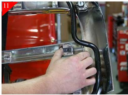
Place supplied U-Clips on the just drilled locations as shown above.
