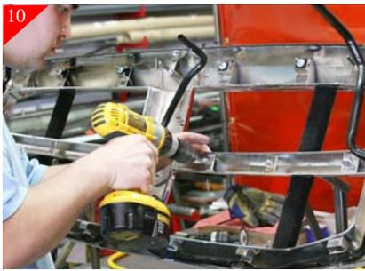
After marking hole locations remove the billet grille . Then using a 3/16" drill bit, drill in the just marked locations.
