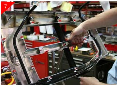
Using a cut off wheel or a pair of dykes cut or remove all the clips that held stock centers as shown above in "RED".
