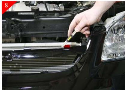
8 Locate the (2) outer tabs one on the drivers and one the passenger side on the top section of the stock grille shell shown above in "RED". Using a utility knife cut the tabs off so as they won't hit the billet grille when it is installed.
