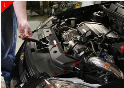
1 Remove (8) plastic push pull rivets from across the top of plastic shroud covering core support. Shown above in "RED". Top portion of plastic will be free at this point.
