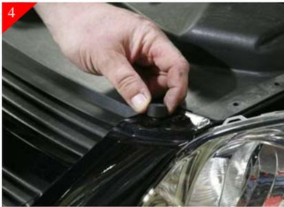
4 Remove the rubber hood bump stops as shown above. You will need to save rubber stops as you will re-install them a little later in the install.
