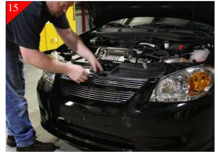
Place the plastic shroud that covers the core support area, go ahead and put in a couple of the plastic push pull rivets to hold in the correct place for marking of the holes in the top brackets.
