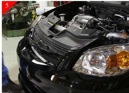
5 Release plastic clips from backside of grille shell by pushing over to release. There are (6) clips surrounding the shell and (4) clips located in the middle of the grille shell. Center plastic portion of grille shell will be free. As shown above.
