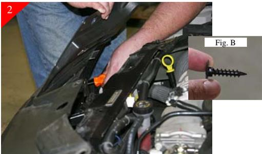
2 Remove plastic Phillips head screws from the backside of the stock grille shell. Screws are located about headlight height. See (Fig. B.) for a detailed photo of the stock screw that is to be removed.
