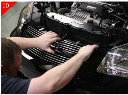
Place u-clips on the bottom brackets with the u-clips going on the "Short" end of the brackets. Then place u-clips on the top brackets with the u-clips going on the "Short" end of the brackets. Then attach both the upper and lower brackets to the billet grille using the supplied #8 x 5/8" Phil pan head screws. After attaching brackets place billet grille into opening from the backside and center.
