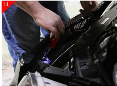
Place billet grille back in opening and attach bottom portion of billet grille to the just placed u-clips using #8 x 5/8" Phil pan head screws as shown above.
