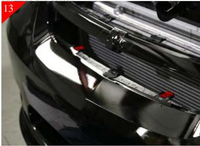
Place the supplied u-clips on the just drill locations as shown above in "RED".
