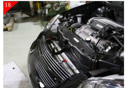
Place the supplied u-clips on the top brackets as shown above in "RED". Then replace the plastic shroud and all the plastic push pull rivets.
