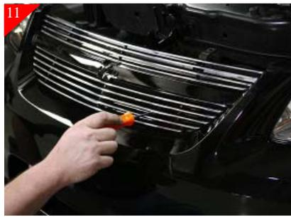
Using a 90° scribe mark the hole locations for the bottom brackets as shown, then remove billet grille.
