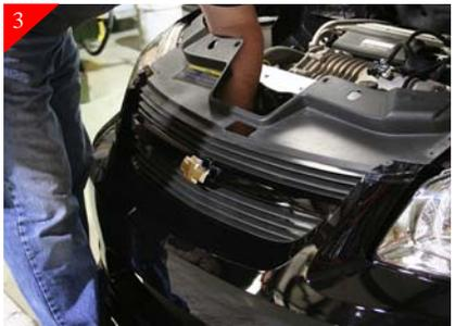
3 Remove the stock "chevy emblem" by removing (2) 10 mm. Nuts from the backside of the emblem.
