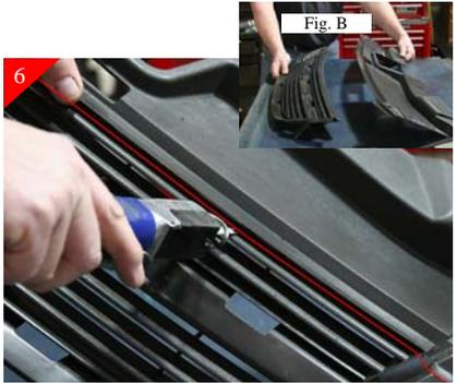
6 Trim the plastic that was removed in the previous step by following along the "RED" cut line shown above. You will be using the top portion of the trimmed plastic only. (Fig. B) shows completed cutting with top and bottom separated.
