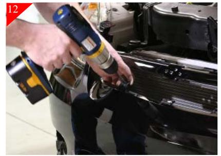
Using a 3/16" drill bit drill in the just marked locations.
