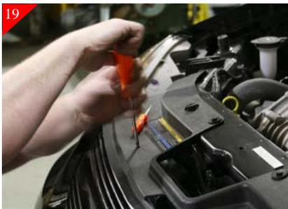
Attach the top brackets to the plastic shroud using the supplied #8 x 5/8" Phil pan head screws and as shown above.
