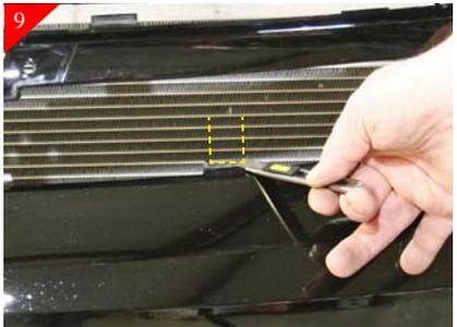
9 Locate the (2) outer tabs on the bottom section of stock grille shell. You will need to notch the backside of the tabs as shown. This allows the new brackets to lay flat in the notched locations.
