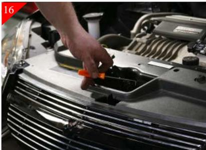
Reach thru the hood release opening and use a scribe to mark the hole locations where the top brackets meet the plastic shroud. After marking remove the plastic shroud.
