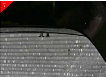
After attaching the brackets replace the plastic rivets that were removed in step 4.
