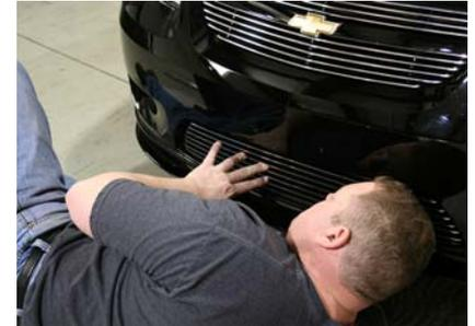
Using a 90° scribe reach up from under front end of vehicle and mark the hole locations in brackets. After marking remove the billet grille from opening.
