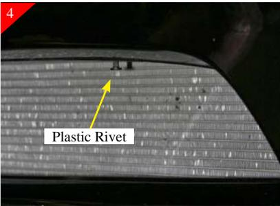
Located and remove the (2) plastic rivets in bumper opening before drilling. This allows you to pull the plastic down making it easier to drill and also so as to not hit anything during the drilling process.
