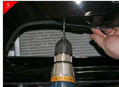
Drill a 3/16" hole in each of the marked locations as shown above.
