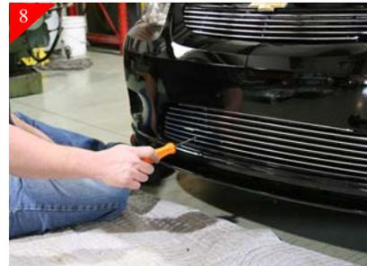
Place billet grille back in opening and center and then attach billet grille to brackets using #8 x 5/8" phil pan head screws as shown above.
