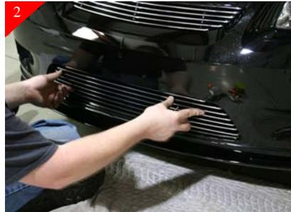
Place billet grille into opening and center. There is a raised ridge in bumper opening, the brackets should butt up against the ridge.
