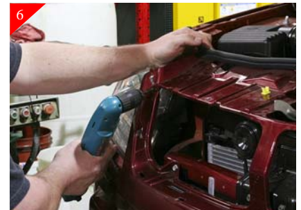
6 Remove stock chome section from vehicle. Then using a 3/16" drill bit, drill in the just marked locations. Note: Pull out on shell, this will allow you to drill without hitting anything.
