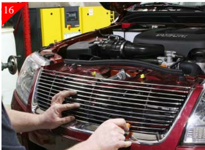
16 Attach billet grille to brackets using the supplied #8 x 5/8" Phil pan head screws.
