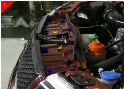
1 Open hood and remove (8) plastic rivets located across the top of the core support shown above in (Blue).
