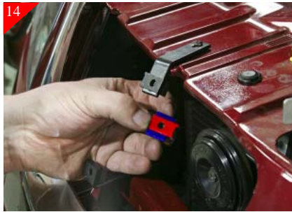
14 Attach bottom brackets to U-clips located on bottom of grille shell opening (Ref. step 13 Blue) using supplied #8 x 5/8" Phil pan head screws. Attach top brackets using the square tabs (Ref. step 13 Green). Square tabs go on the underside and attach using #8 x 5/8" Phil pan head screw as shown above.
