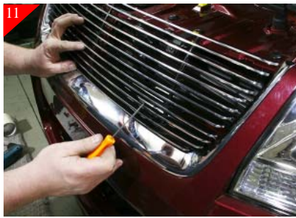
11 Place the billet grille into the opening and center. Using a 90° scribe reach thru the front of the billet grille and mark the holes in the bottom brackets as shown above. Then mark the holes for the top brackets. After marking remove brackets from billet grille
