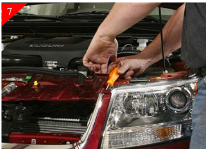
7 Re-place the chome section. Then attach chome section using the supplied #8 x 5/8" Phil head screws in the just marked locations as shown above. NOTE: Just snug the screws up--Do Not Over-tighten.
