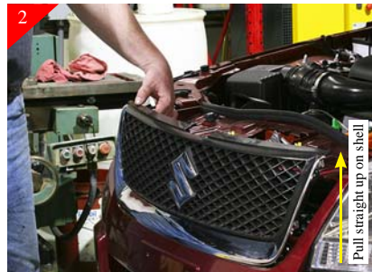
2 Starting with the drivers side corner of vehicle, pull straight up on the stock grille shell to release. Then repeat for the passenger side. Grille shell will be free at this point.
