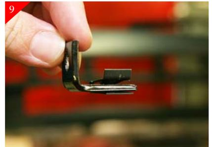
Place supplied U-clips on the long end of the supplied brackets as shown above. Attach brackets to billet grille using the supplied #8 x 5/8" Phillips pan head screws. With brackets attached place billet grille into the opening and center.
