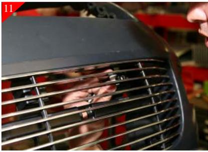
Next place the supplied spacer between the billet grille and the shell, then place the supplied 1/4-20 x 3/4 soc head bolt into hole. This will hold the spacer in place while marking the bottom brackets for drilling. Now mark the hole locations for the bottom brackets where it meet the shell.
