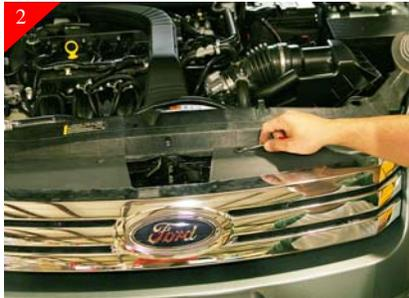
Remove plastic rivets across top of core support. A small regular screwdriver will aid in removing.
