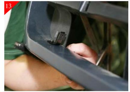
Remove the bottom brackets from billet grille and attach them to the shell. Using the supplied 1/4-20 x 3/4" Soc head bolts and 1/4-20 nuts as shown above.
