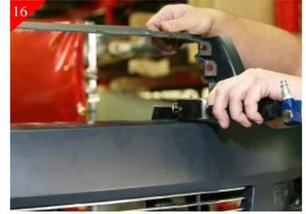
Using an air saw or hack saw remove the center of the grille shell as shown.
