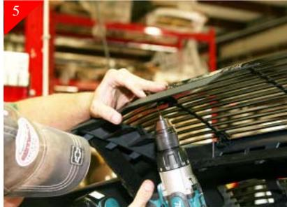
Place billet grille into opening and center. Mark the hole locations for the top brackets where it meets the stock shell. Repeat for the bottom brackets. Drill a 3/16" hole in each of the just marked locations.
