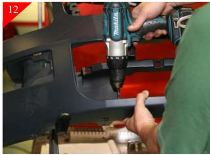
Remove the billet grille from opening and using a 3/16" drill, drill in the just marked locations as shown above.
