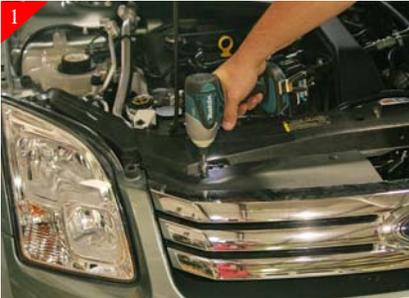
Remove (2) 10mm bolts from along top of stock shell.
