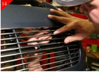
With the bottom brackets attached place the billet grille back into opening and center. Place the spacer between the billet grille and the shell (Ref. step 11), then attach using the supplied 1/4-20 x 3/4" Soc head bolts and 1/4-20 nuts
