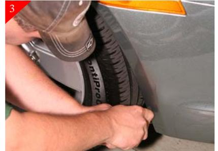
Now Locate (3) per side in wheel wells plastic rivets & remove.
