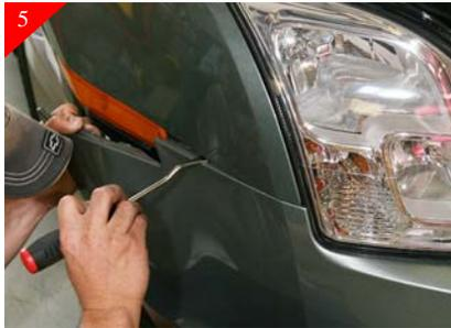
Starting on either side of the vehicle. Using a pry tool or screwdriver. Release the clips holding front end in place. Push pry tool in and lift up on the clip to release.
