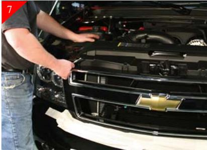
7 Remove (6) 10mm. bolt from along core support area. This will allow you to reach behind the stock shell.
