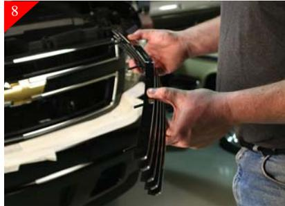
8 Place the supplied bolts in bottom billet grille as shown above. Then place billet grille into opening and center.
