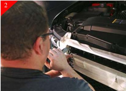
2 Remove the "Egg Crate" section by using a pair of dykes to snip out as shown above. You are just removing the bulk of the "egg crate" section as much as you can.
