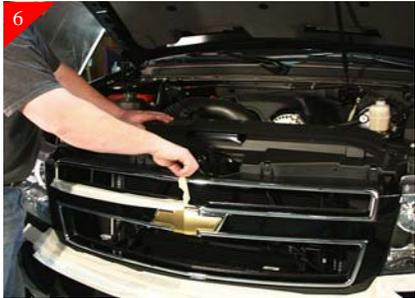
6 After sanding remove the masking tape from stock shell, leaving tape along bumper as shown.
