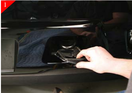
1 Remove the rubber surrounding tow hooks, by pushing straight back to release.
