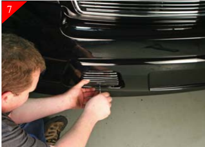
7 Now attach billet grilles to the just attached brackets as shown above.
