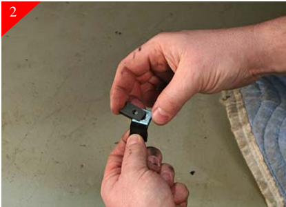
2 Place the supplied U-clips on the supplied brackets as shown above.
