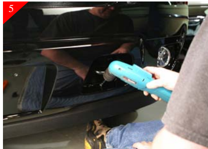
5 Remove the billet grille from opening and also remove the brackets from the billet grille. Then drill a 3/16" hole in each of the just marked locations.
