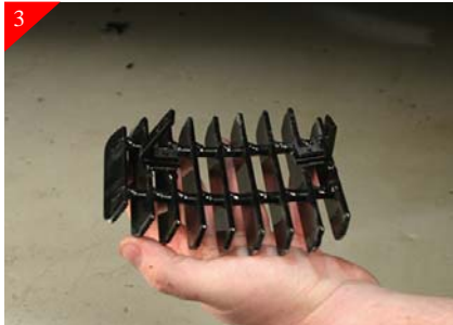
3 Then attach brackets to billet grille using the supplied #8 x 5/8" Phil pan head screws as shown above.
