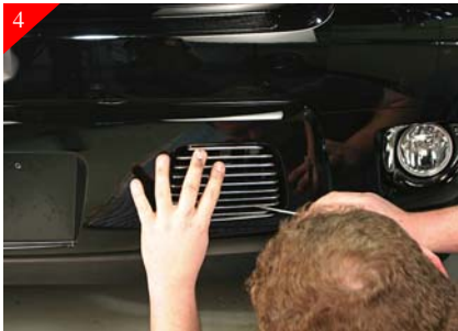
4 Place billet grille into opening and center. Then using a 90° scribe mark the location of the holes in bracket where it meets the vehicle.
