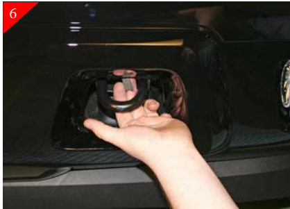
6 Now attach the brackets to the just marked locations. Attach the top bracket by placing a supplied u-clip on the top side of the tow hook opening as shown above then attach brackets to uclip using #8 x 5/8" Phil pan head screws. Repeat process for the bottom brackets.
